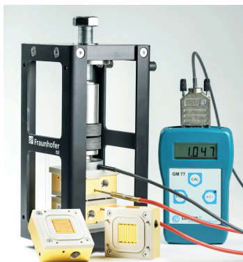
Gold-coated PEM electrolysis test cell with temperature sensors and force sensor for adjusting the clamping pressure.
