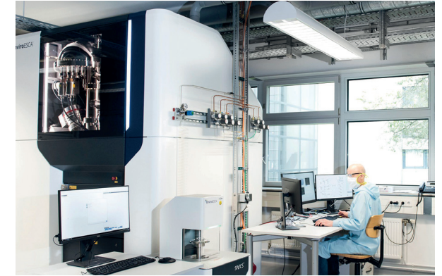
The HT-NAP-XPS system of Fraunhofer ISE provides high measurement performance for material characterization.
