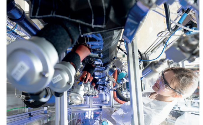
Distillation column with a total height of 7.5 meters for developing an industrial scale synthesis of dimethyl ether and other sustainable energy carriers.
