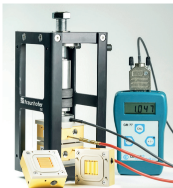
Gold-coated PEM electrolysis test cell with temperature sensors and force sensor for adjusting the clamping pressure.
