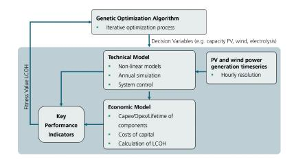
Schematic layout of the model structure in  $H_2$ ProSim for the least-cost optimization of the system. Fraunhofer ISE models, simulates and optimizes hydrogen systems.
