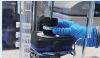
4 Analysis of ink homogenisation processes to break up agglomerates
