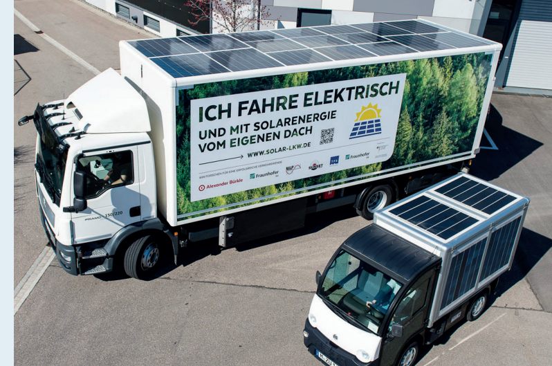
Electric-powered truck and mini truck, both with integrated photovoltaic modules.
