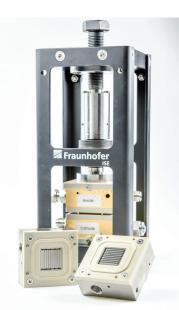
For our customers and partners we offer our standard 4cm<sup>2</sup> electrolysis test cell. Worldwide it is already used by various working groups for numerous measurement tasks. © Fraunhofer ISE
