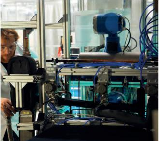
Measurement of air temperature and humidity in the climatic chamber.
