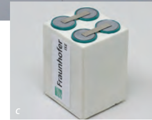
c: PCM composite for thermal management of batteries; d: Thermal energy storage tank in demonstration plant.
