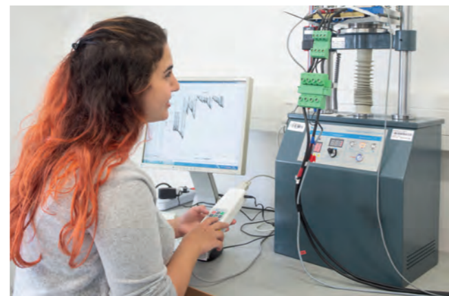
Press for the controlled compression of pouch cells. © Fraunhofer ISE/Photo: Dirk Mahler
