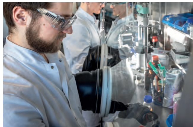
Glovebox for preparation of sulfide-based solid-state batteries. © Fraunhofer ISE/Photo: Dirk Mahler
