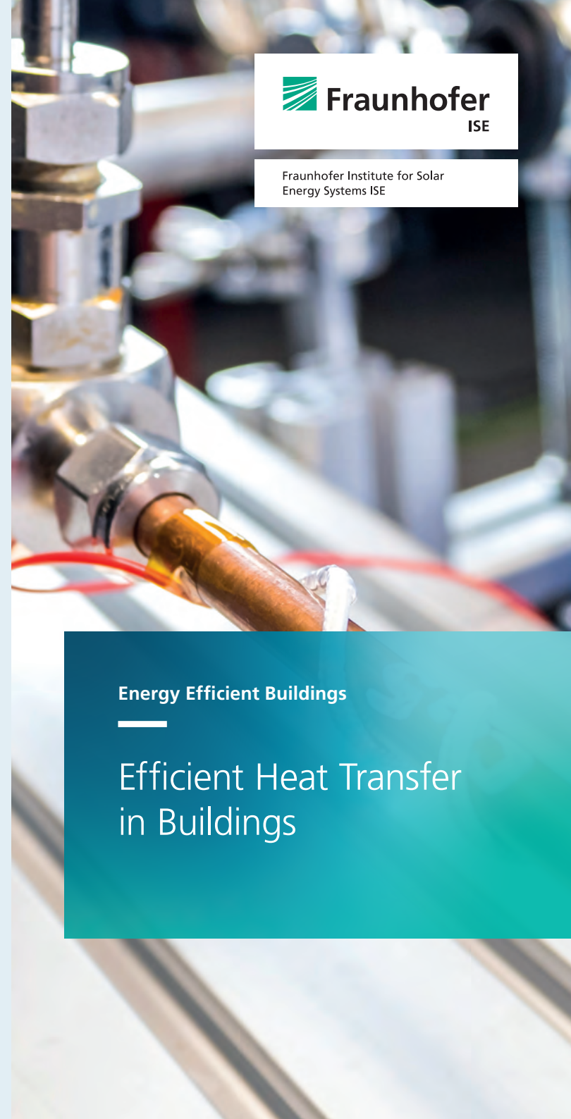
Cover photo: Bake-out of a heat pipe during the evacuation process.
