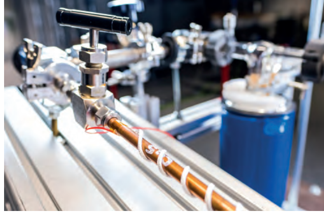
Evacuation and filling of a heat pipe according to customer-specific requirements.
