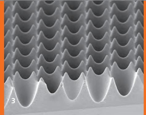
3 SEM image of a hexagonal grating fabricated via interference lithography. This grating has a period of  $8 \mu\text{m}$  and a height of  $9 \mu\text{m}$ .
