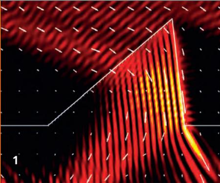
1 Near field calculation of a micro prism array. The color scheme shows the intensity distribution, the white arrows depict the Poynting vectors.
