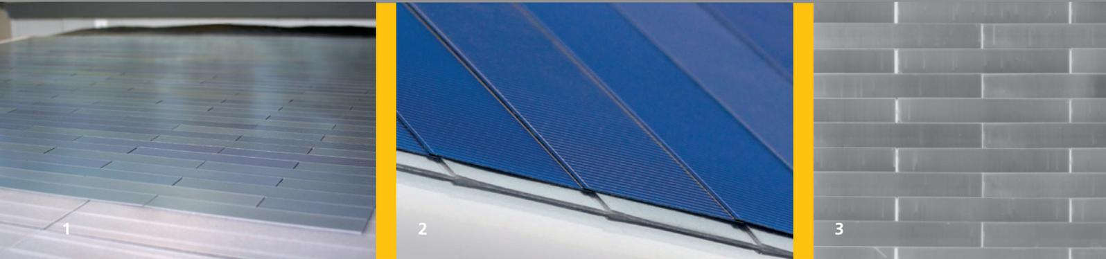
1 Production of a shingle module in matrix technique with pSPEER solar cells at Module-TEC, Fraunhofer ISE.
