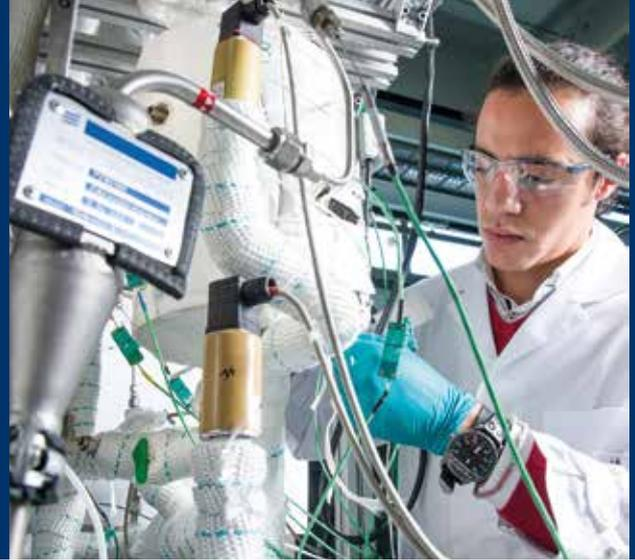
*Detail of a mini-plant at Fraunhofer ISE to produce methanol and dimethyl ether (DME) from carbon dioxide and hydrogen.*
