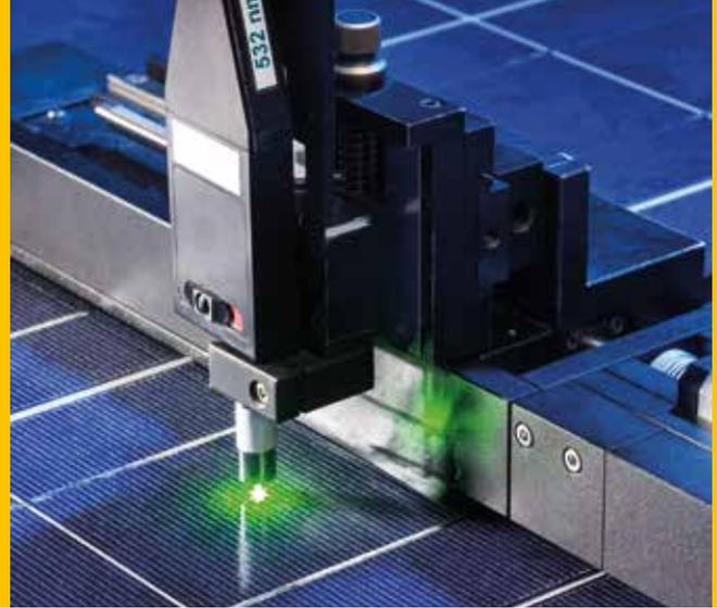
*Non-destructive material analysis for PV modules applying Raman spectroscopy. This technology is used to determine the spatial distribution of degradation behaviour due to the polymer encapsulation material of PV modules. It allows degradation indicators for lifetime models to be measured simply and aging mechanisms to be identified.*
