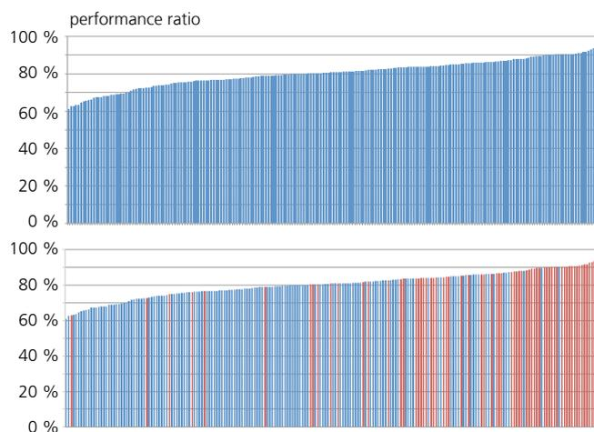
2 Annual benchmarking exercise for the Performance Ratio of 300 PV power plants based on performance in 2014. In the bottom graph the red lines indicate power plants subject to quality assurance by Fraunhofer ISE.
