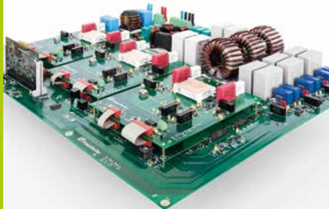
*Three-phase PV inverter for use in the laboratory. The modular design allows the most modern circuit topologies and semiconductor modules to be tested efficiently. New control algorithms can be investigated under realistic conditions and optimized using the digital signal processor and extensive measurement data acquisition.*
