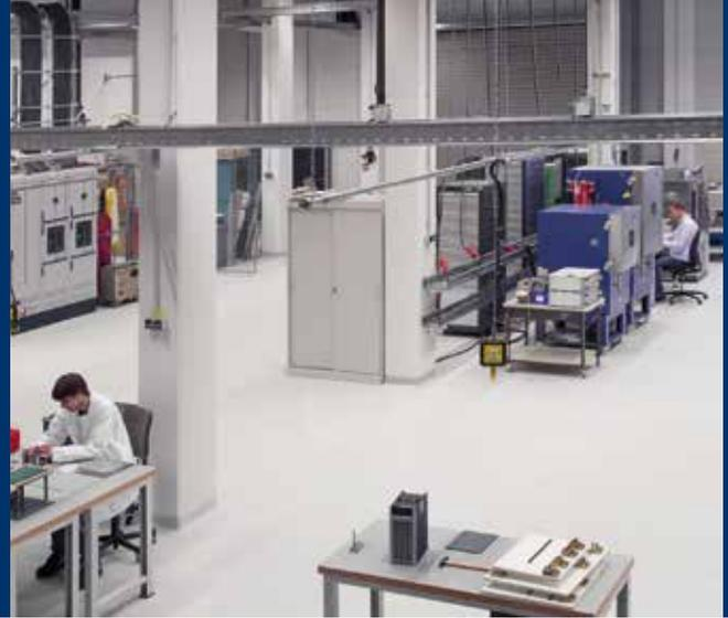
*Interior view of the ServiceLab Batteries at Fraunhofer ISE. It is equipped with extensive testing facilities for cells, battery modules and complete systems of up to 1000 V and 0.25 MW.*
