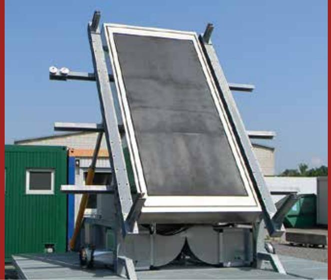
*Outdoor test Facility for Real-size building Envelope Elements (OFREE) with an area of up to 4 m x 3.77 m (shown here without a façade element mounted). The black calorimeter absorber surface is clearly visible, as are the I-profile rails of the tracker, on which the rectangular calorimeter is mounted. The ventilation unit for a well-defined external heat transfer coefficient is installed after the façade element has been mounted.*
