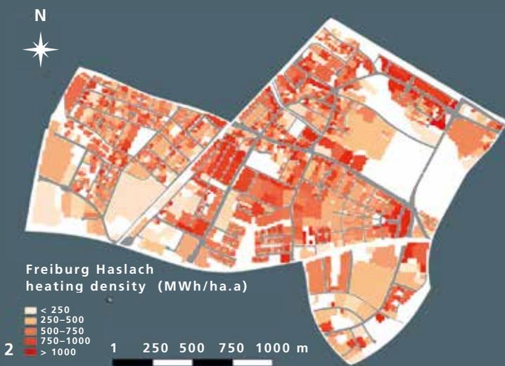
2 "Energiequartier Haslach": Based on the density of the heating demand and electricity load profiles, supply scenarios for heating and electricity are developed and optimised. When combined with the potential of renewable energy sources, suitable locations for storage units can be identified.
