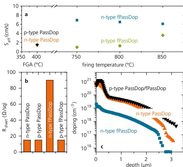
2 Properties achieved with the PassDop process on n-type and p-type surfaces: a) Passivation quality as a function of subsequent firing temperature; b) Sheet resistance of the local doping; c) doping profiles of the local doping.
