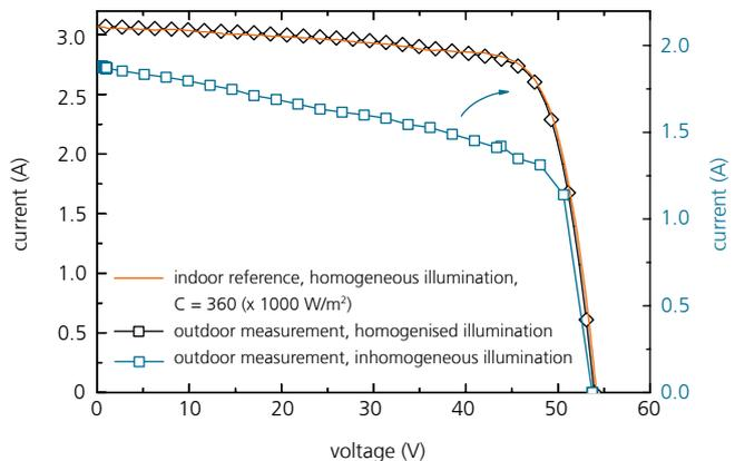
2 Current-voltage characteristics of a concentrator module with a reflective system under homogeneous illumination indoors, outdoors with “homogenising” optics and outdoors without the homogenising component. In contrast to homogeneous illumination, inhomogeneous illumination causes losses due to spillover beyond the edges of the receiver and mismatch losses in the fill factor due to the series connection of solar cells on the receiver.
