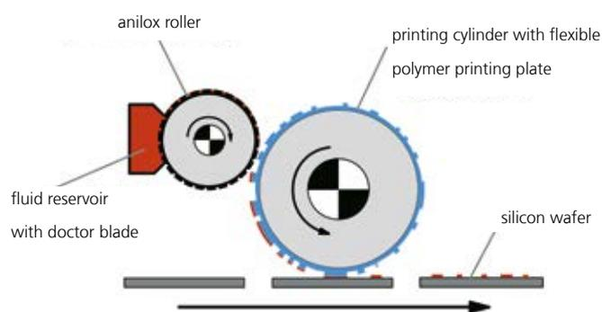
**3** Schematic diagram of the flexography process: An engraved anilox roller transfers a defined volume of printing fluid onto a flexible plate around the printing cylinder and from there directly onto the silicon wafer.
