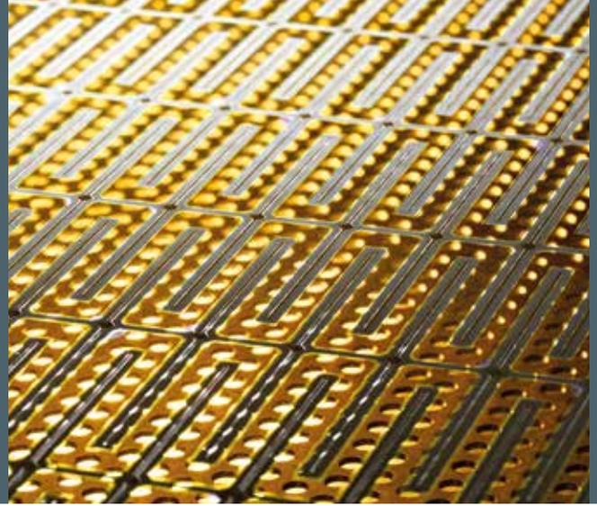
*Detail from the production of a dye solar module sealed with glass frit.*
