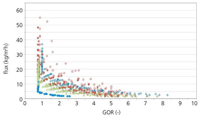
**2** Simulation results for widely varying MD module configurations, which indicate the opposing directions for optimising energy efficiency – characterized by the degree of heat recovery (GOR) – and area-specific productivity – characterized by the flux. The simulation allows the application-specific optimum to be determined.
