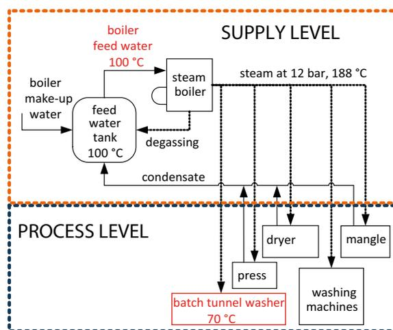
2 Laundry with its steam network and processes. The steam generated by the boiler is supplied directly to the applications or via heat exchangers. The integration processes for solar process heat, which were investigated as examples, are marked in red.
