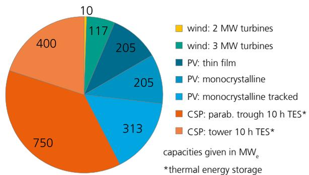
2 Distribution of renewable energy technologies in the Shagaya energy park based on the simulations for the optimisation study. The primary goal resulting in this mix was electricity supply during peak load periods.
