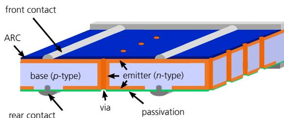
5 Structure of the BSK solar cell (“BSK” is from the German “beidseitig sammelnd und kontaktierbar”, referring to a double-sided emitter and contacts on either side).
