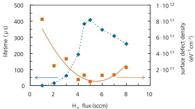
2 Charge carrier lifetime and defect density of sputtered aluminium nitride versus hydrogen flux determined during deposition. Coating of p-type, 1 Ωcm FZ wafers. After further process optimisation, values exceeding 1000 μs were achieved (not shown here).
