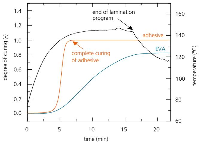
2 Simulated curing of a conductive adhesive and EVA.
