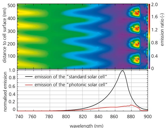
2 Above: Ratio of the depth-dependent emission from the photonic solar cell to that from a "standard solar cell". Below: Total emission from a photonic solar cell in comparison to a "standard solar cell". The reduction in emission is evident.
