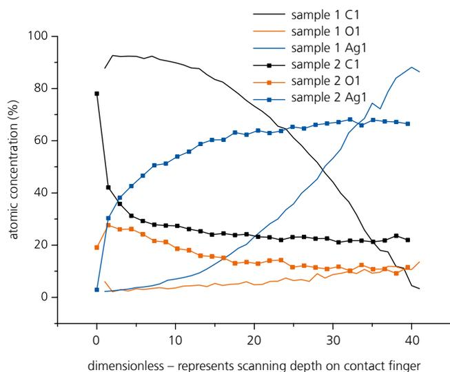
3 Concentration depth profiles from the Auger spectroscopic investigations on extracted contact fingers. For sample 1, the oxygen concentration increases with the silver concentration, which is interpreted as an indication of silver oxide formation. The second sample does not confirm this hypothesis. An elevated oxygen signal is also evident here, which decreases together with the carbon signal from the encapsulation material.
