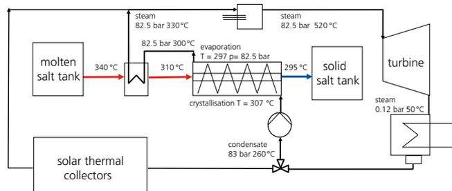
3 Night operation of a 50 MW direct steam-generating power plant with two storage tanks and additionally installed fossil-fuelled auxiliary burner during tank discharging.
