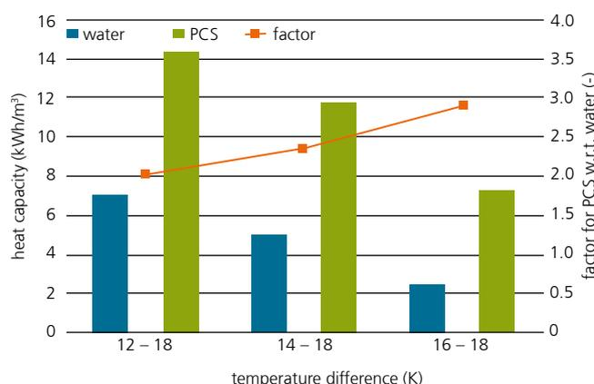
**3** *The PCS offers a significantly higher storage density than water. This means that storage units can be dimensioned smaller for the same heat capacity. The smaller the usable temperature difference, the greater is the advantage of PCS compared to water.*
