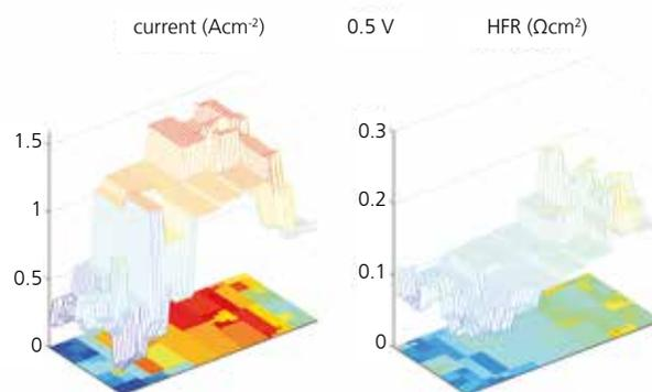
**2** *(left) The current density distribution of a 200 cm<sup>2</sup> cell reveals low current generation near the gas inlet and the gas outlet, for measurements made with a cell voltage of 0.5 V and a stoichiometry of 2.2 : 2.3 (H<sub>2</sub> : air). (right) The locally measured high-frequency resistance (HFR) identifies membrane dehydration and thus raised ohmic losses near the gas inlet.*
