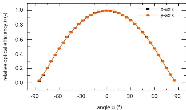
3 Ray-tracing results for the relative optical efficiency value including the cosine losses versus the angle of rotation around the x and y axes. No visible effects of reflection due to the frame are visible.
