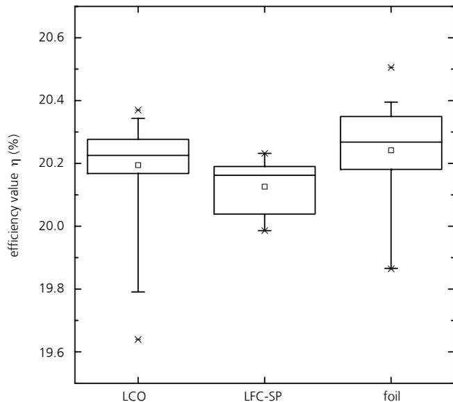
2 Efficiency values of PERC solar cells produced by industrially relevant processes. The cell with a foil electrode presented here (foil) is compared with commercially established processes to produce local back contacts on the basis of screen-printed electrodes – LCO (local contact opening) and LFC-SP (laser fired contact, screen-printed). Each group of results is based on 15 to 41 solar cells which were produced from magnetically grown Cz silicon with identical front cell surfaces.
