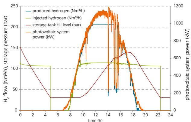
2 Dynamic behaviour of a PtG system with a pressurised PEM electrolyser which responds to the power profile (orange) of a photovoltaic system. The generated hydrogen (blue) is temporarily stored under pressure (red) and injected into a natural gas pipeline (green) as required. For clarity, only a constant injection capacity is assumed.
