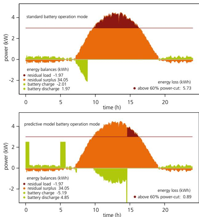
2 Generation and load data for a typical private building. Prediction-based algorithms have been developed to buffer the power peaks.
