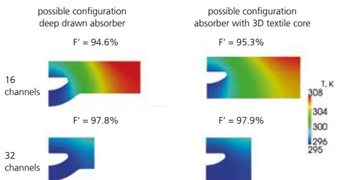
2 Temperature distribution and collector efficiency factor  $F'$  for different examples of channel configurations (stationary). The number of channels refers to an absorber width of 1 m. The interior channel height is 4 mm.
