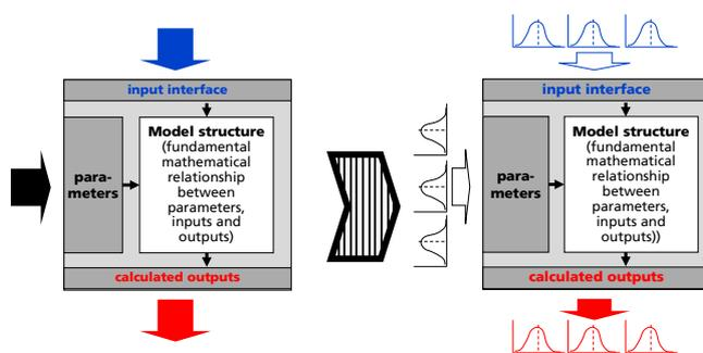
3 Procedure for simulation or optimisation under uncertain boundary conditions. Some or all parameters and inputs are described by probability distributions. The result is a probability distribution for the outputs, which allows a concept to be evaluated.
