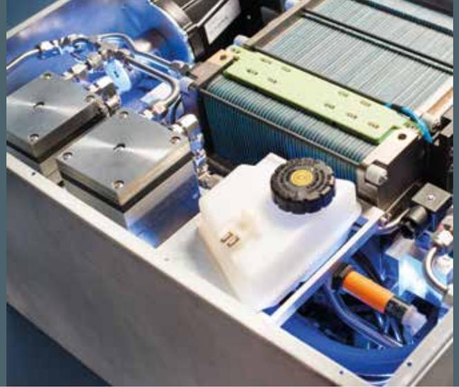
*Hydrogen-based fuel cell system with an output power of 1.5 kW for seasonal energy storage.*
