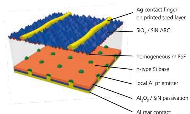
2 Schematic representation of our n-type Si solar cell with back-surface Al emitter points. The well-known PERC technology for p-type cells can be applied for n-type cell production without essential changes.
