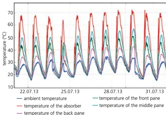
3 Change in temperature with time for the different collector layers.
