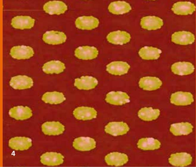
4 Atomic force microscopy image of elliptical silver nano-particles to exploit plasmonic effects in solar cells. The particles can be produced in a well-defined form over a large area by a processing chain consisting of interference lithography, nanoimprint lithography, metallisation and lift-off. The particles have semi-major and semi-minor axes of 120 nm and 70 nm respectively, and are arranged hexagonally with a lattice plane separation of 300 nm.
