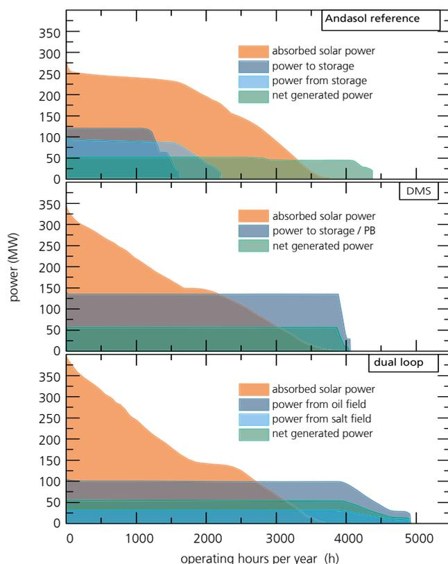
Fig. 2 presents the power versus the operating hours per year for the reference, DMS and dual-loop power systems located in Daggett, USA. The lowest LCOE for the assumed parameters is achieved with the dual-loop concept. The direct molten salt concept also achieves low LCOE, is less complex and is best suited to providing power flexibly. If the costs of the solar field and the heat exchanger system could be reduced by about 15%, the direct molten salt concept could present the best option.
