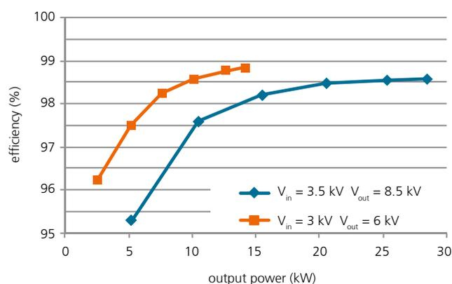
3 First measurements show a maximum efficiency value of 98.5% for the rated power of 28 kW. Still higher efficiency is achieved for a lower output voltage and a lower duty cycle.
