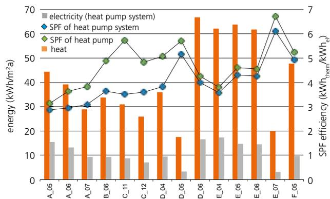
2 Results of analysing monitored data from large heat pump systems in non-residential buildings: heat provided, electricity consumption of the heat pump systems, seasonal performance factor (SPF) of heat pump (compressor only) and SPF of heat pump system (heat pump and primary loop).
