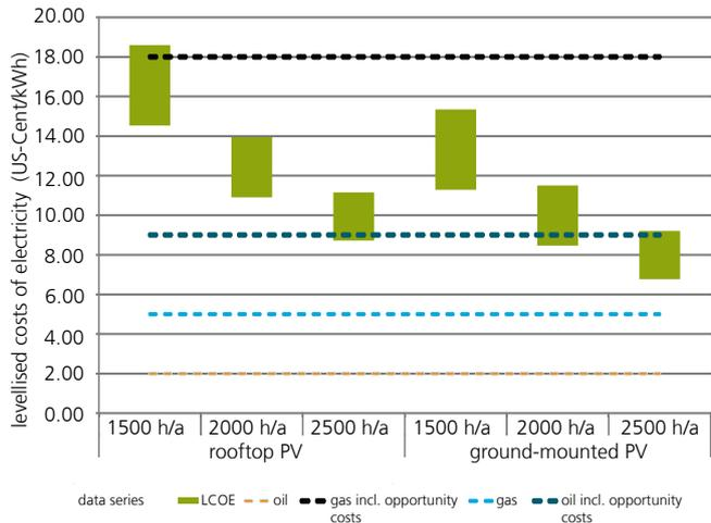
2 Comparison of the levelled cost of electricity (LCOE) for PV systems and conventional technology with opportunity costs.
