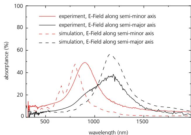
5 Polarisation-dependent measurement and simulation of the absorbance spectra of the elliptical silver nano-particles on glass illustrated in Fig. 4. The polarisation directions are oriented parallel to the semi-axes of the particles. In this case, rigorous coupled wave analysis (RCWA) was used as the simulation method in order to reproduce wave-optical plasmonic effects.
