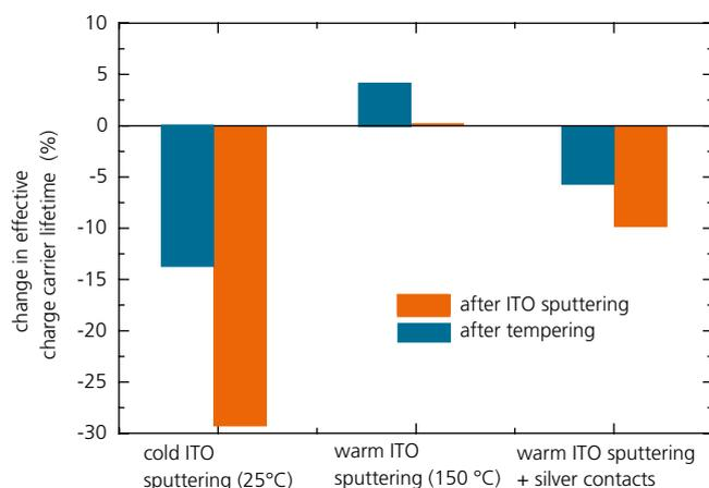
**2** Relative change in the effective charge carrier lifetime, measured for silicon wafers that were bifacially passivated with Si layers, directly after the ITO sputtering processes and after tempering in air at 150 °C for 12 minutes.
