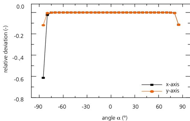
2 The relative deviation of a LARC® with a frame compared to one without a frame shows the shading of the cell by the frame for different angles of rotation around the x and y axes.
