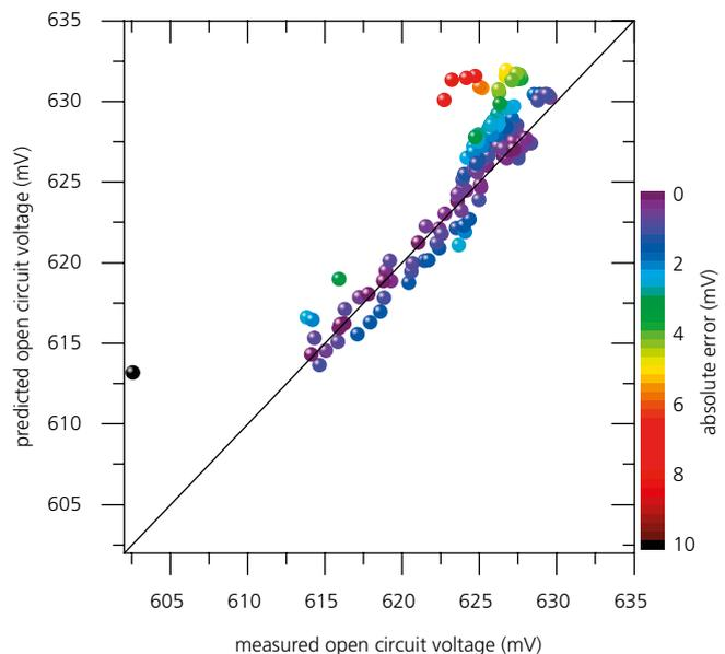
2 Applying the procedure of Fig. 1, prototypical characteristics were extracted from PL images of untreated wafers and used to train a model to predict the open circuit voltage. The graph shows the prediction result for the open circuit voltage of 164 wafers from three bricks of an unknown block. The small relative deviation of less than 0.3% on average demonstrates the suitability of the procedure.
