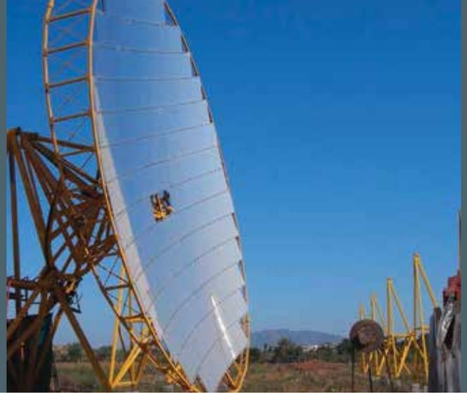
*Scheffler reflector to generate steam to drive a 1 MW turbine using waste heat in Rajasthan, India.*
