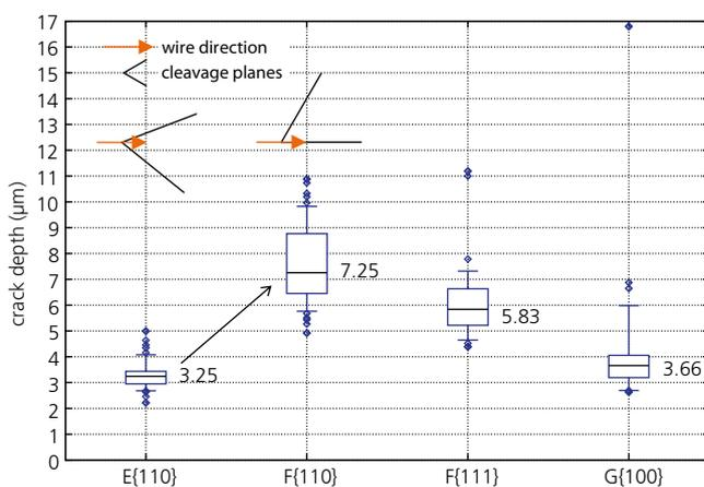
3 Maximum crack depth as a function of surface crystal orientation for a multicrystalline silicon wafer.
