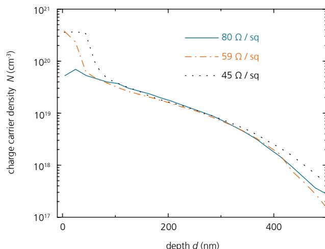
2 Different phosphorus doping profiles created in co-diffusion processes and the associated sheet resistance. The phosphorus doping profile of the BSF can be deliberately adjusted without changing the boron doping profile of the emitter.
