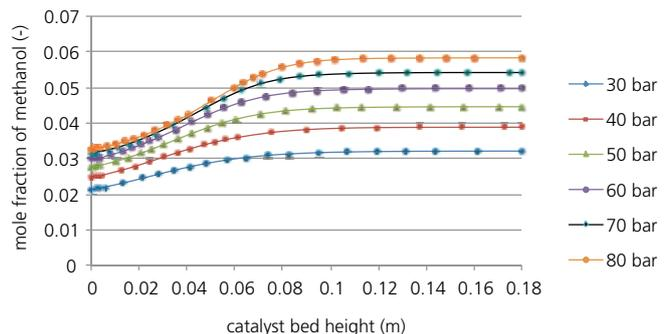
2 Results of the Bussche-Froment simulation of one of the two reactors. As the methanol synthesis is based on a volume-reducing reaction, the methanol fraction increases with increasing pressure. The simulation also shows that the equilibrium concentration is already reached at a catalyst bed height of 0.1 m and that no further reaction occurs in the second half of the reactor (which could thus be dispensed with).
