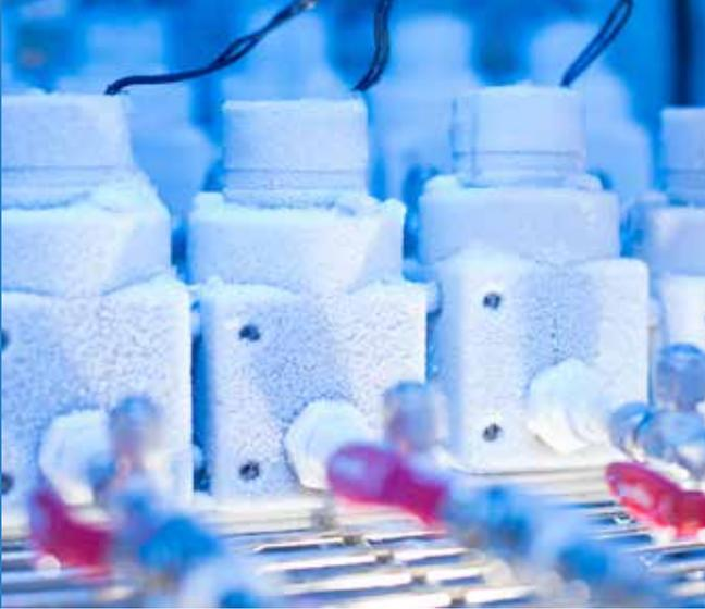
*Long-term test of valves at low temperatures in a test cell integrated into a climatic chamber .*
