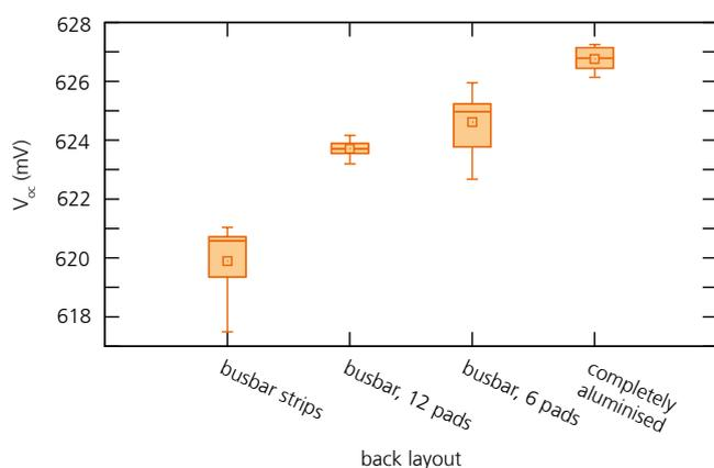
2 Comparison of back busbar layouts:  $V_{oc}$  gain by layout adaptation.
