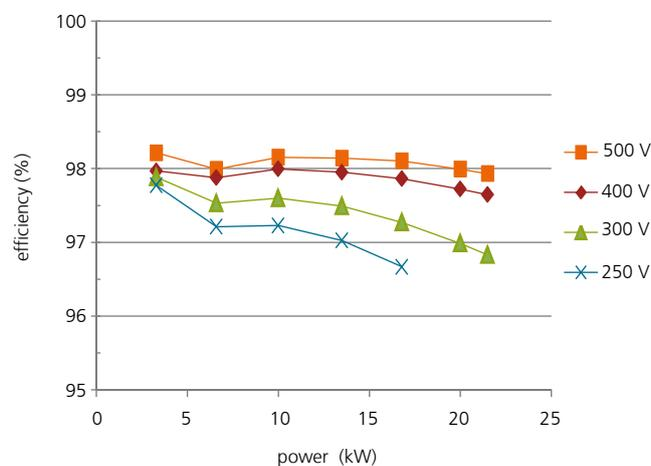
2 Efficiency of the bidirectional charger for different battery voltages and powers.
