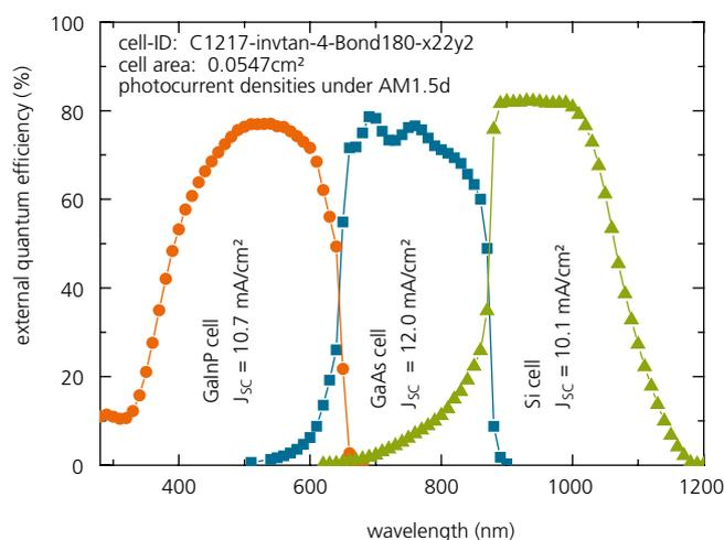
3 External quantum efficiency of a GaInP/GaAs/Si triple solar cell. The photocurrent densities were calculated for each sub-cell at AM1.5d.
