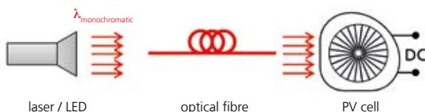
**3** Schematic configuration of a system for optical energy transmission. A laser serves as the optical energy source; its monochromatic radiation is transmitted via an optical fibre onto a photovoltaic cell. This converts the optical energy with high efficiency into electricity.
