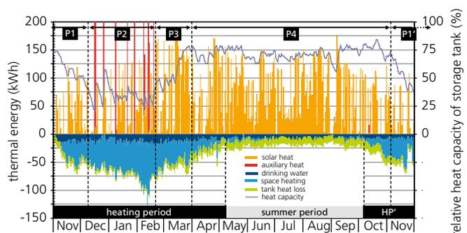
2 Characteristic operating phases of a Solar-Active-House with a solar-thermal fraction of about 70%. The graph shows the thermal gains and consumption (left-hand axis) and the thermal capacity of the storage tank (right-hand axis).
