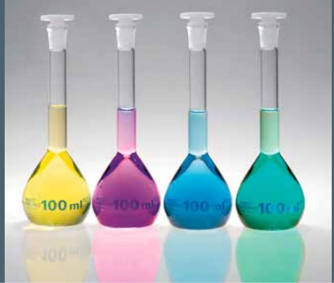
The four oxidation states of the diluted vanadium electrolyte (from left to right:  $V^{5+}$ ,  $V^{2+}$ ,  $V^{4+}$ ,  $V^{3+}$ ).
