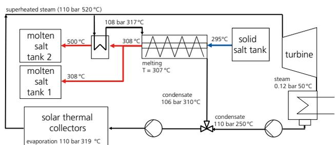
4 Daytime operation of a 50 MW direct steam-generating power plant with three storage tanks during tank charging.
