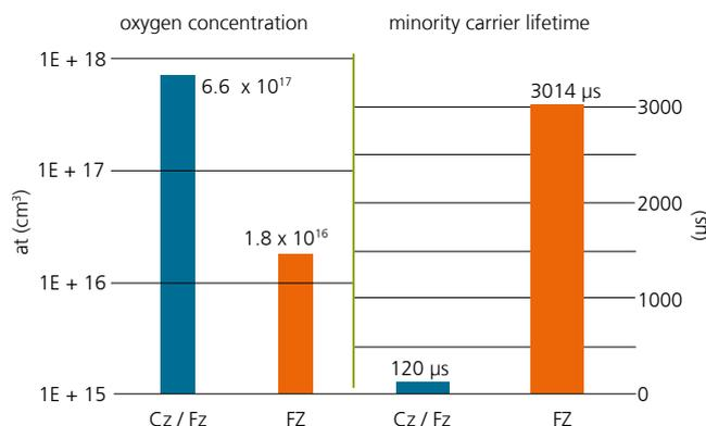
2 Oxygen concentration and minority carrier lifetimes in pre-formed feed rods (blue) and the 4" FZ crystals (orange) produced from them. The oxygen concentration can be reduced by more than an order of magnitude, the carrier lifetime increases by a factor of 25. Oxygen detection: FT-IR (CIS, Erfurt); lifetime: QSSPC (quasi-steady-state photoconductance) (CSP-ZTN Halle).
