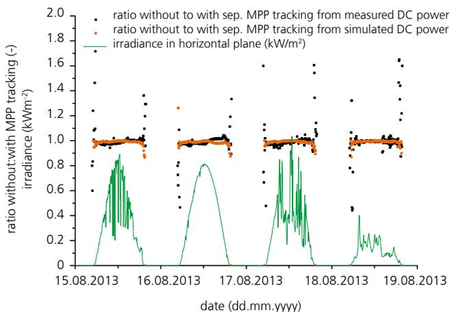
3 Ratio of the DC power from the system in Ichttershausen for parallel-connected, east/west oriented, vertical module strings without/with separate MPP tracking; black – from measured DC power values, red – from simulated values, green – irradiance in the horizontal plane.
