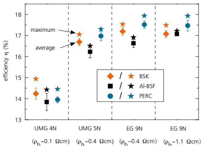
6 Average and maximum efficiency values for BSK, Al-BSF and PERC solar cells of multicrystalline material with different base resistivity values from UMG-Si feedstock of low purity down to 99.99% (4N) and 99.999% (5N) and high-purity EG-Si feedstock (9N). Each cell has an area of 156 mm x 156 mm. All measurements were made on a non-reflective chuck, i.e. bifacial gains have not been taken into account for the BSK solar cells.
