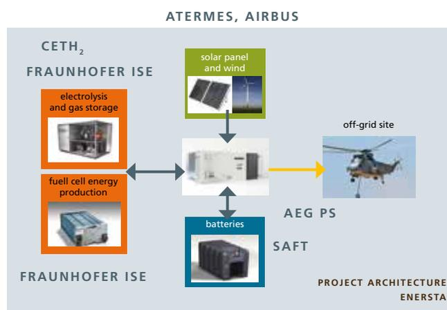
2 Responsibilities of the "Enersta" project partners: AEG is responsible for the overall controls, Saft for the storage battery, CETH<sub>2</sub> for electrolysis and H<sub>2</sub> storage, Atermes for the cabinet, Airbus for the simulation tool and the complete solution and Fraunhofer ISE for the fuel cell system and the H<sub>2</sub> storage.
