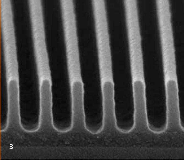
3 Scanning electron microscopy image of a high-frequency linear grating with a large aspect ratio for light-guiding or polarisation-optical applications (period 230 nm).
