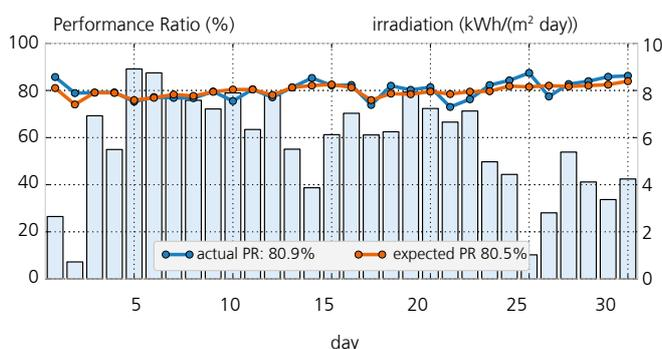
3 Graph comparing the expected and actual PR for a multi-megawatt PV power plant.
