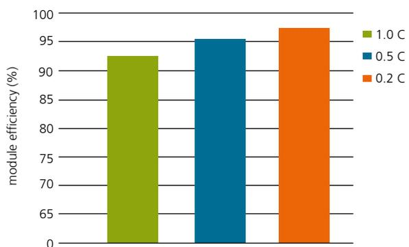
3 *Efficiency values of the lithium-ion battery module for different C-rates (charging and discharging in one hour, two hours and five hours respectively).*
