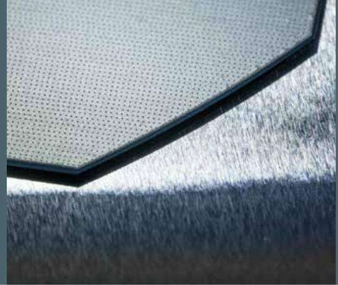
*Crystal silicon solar cell with its aluminium foil electrode.*
