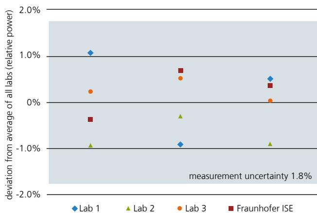
2 The round robin comparison of the four internationally leading calibration laboratories for PV modules demonstrated that the deviation from the average for all participants was  $\pm 1\%$  and thus well within the measurement uncertainty of 1.8% for CallLab PV Modules.
