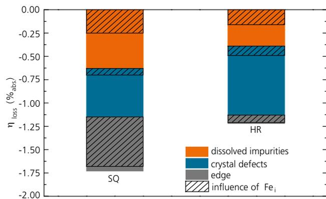
2 Efficiency-Limiting Bulk Recombination Analysis (ELBA) of PERC cells from standard material (SQ) and from material which was produced in extremely pure crucibles (HR). In particular, cells from standard material are limited by diffusion of impurities from the crucible system into the block.
