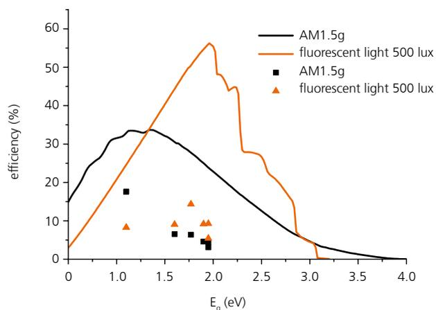
**2** Theoretical (lines) and measured (symbols) efficiency values of different solar cells under illumination by sunlight (black) and a compact fluorescent lamp (red) as a function of the band gap energy of the semiconductor.
