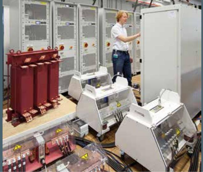
*The Inverter Laboratory of Fraunhofer ISE is equipped with all the facilities needed to test central inverters up to a power rating of 1 MW according to diverse grid feed-in guidelines.*
