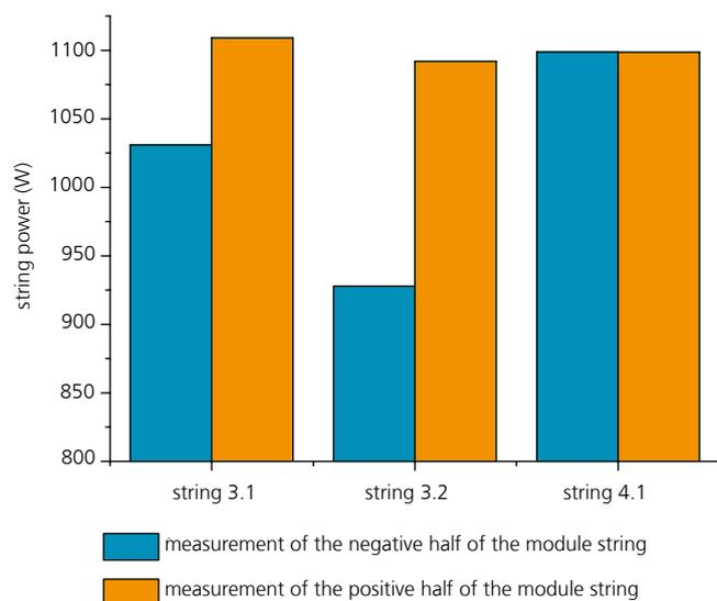
2 Measured power values for half-strings from a plant affected by PID.
