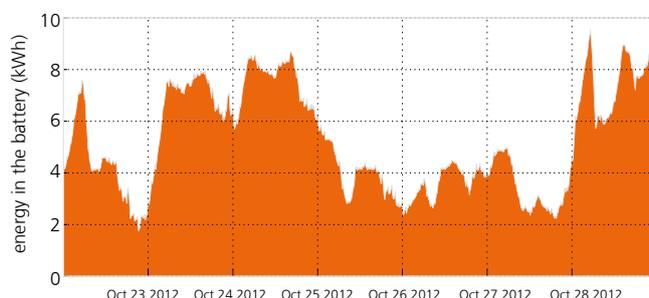
**3 Example of the energy profile for the battery of a free-standing house with a PV system, which not only increases the amount of PV electricity consumed on site but also provides primary control reserve power as a service to the transmission grid operator. The two business models complement each other and enable the battery to be operated economically.**
