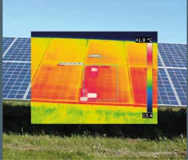
*Thermographic investigation of a solar generator in a photovoltaic power plant. The high-resolution infrared image of a faulty module is superimposed over the digital photo and reveals individual solar cells with noticeably higher operating temperatures. The result is a clear indicator for yield losses and future risks affecting the reliability of the affected module.*
