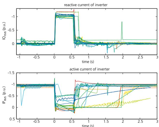
2 Comparison of the active current (below) and the reactive current (above) fed in by various inverters during a three-phase voltage drop to 25% residual voltage ( $t = 0-0.5$  s). The inverters show very similar behaviour with respect to the reactive current. It is problematic that the inverters increase the active current only slowly after correction of the fault.
