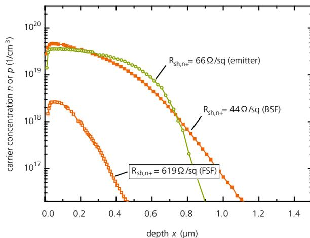
2 Concentration profiles and sheet resistance of the dopants of a BC-BJ solar cell consisting of  $n^+$  back surface field (BSF),  $n^+$  front surface field (FSF) and  $p^+$  emitter. All doped regions were created in a single co-diffusion step. The doping profiles shown here were determined after a further high-temperature step (drive-in).
