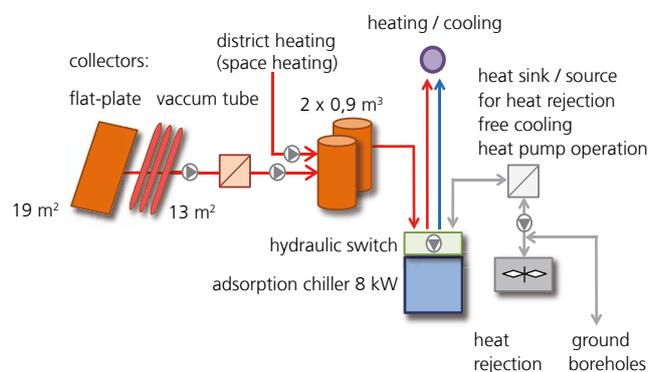
2 Schematic diagram of the solar cooling system at the Technical College. The system is equipped with two different collector arrays for educational purposes. An additional connection to the district heating network ensures that the rooms are heated in winter. The cooling and heating power is distributed via two ceiling-mounted ventilation coolers and a floor heating loop.
