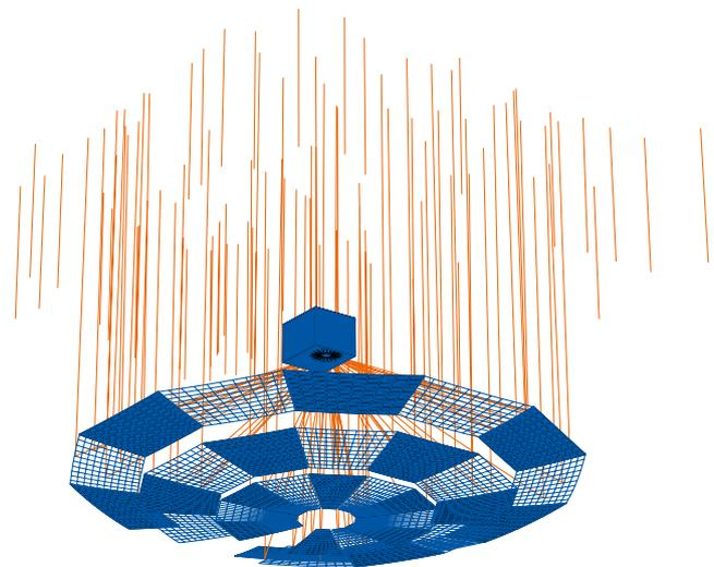
**3** *Dish concentrator for Stirling dish systems: Result of simulation and optimisation with ray-tracing programs.*
