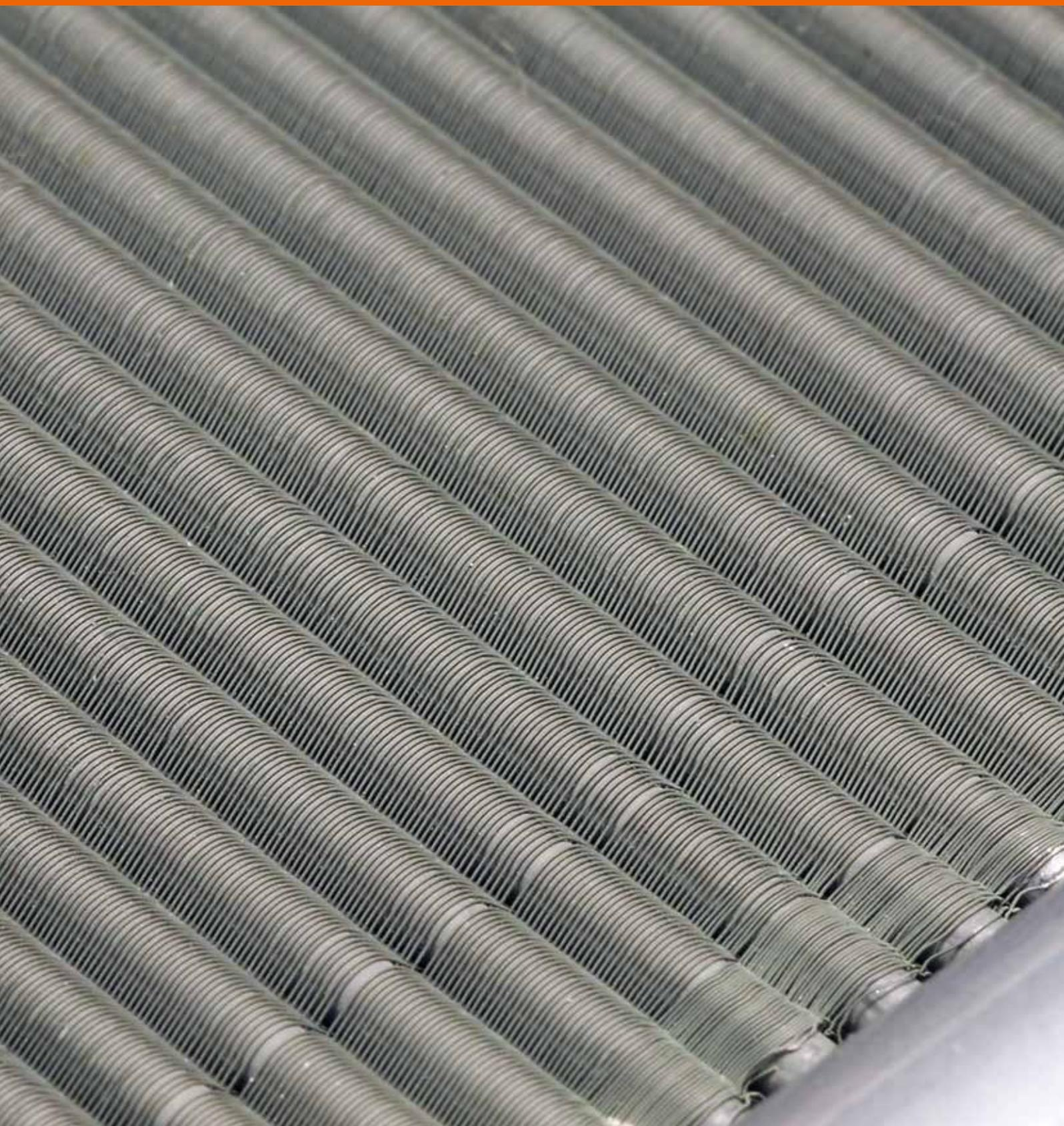
*Macroscopic image of a heat exchanger structure of metal wire mesh for efficient evaporation of natural refrigerants. The prototype has a width of app. 400 mm and a height of app. 100 mm.*
