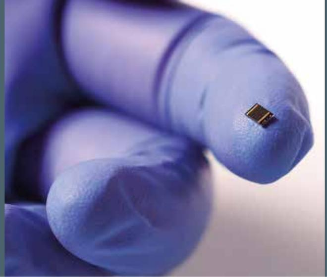
*World record solar cell with an efficiency value of 44.7% (@297xAM1.5d), consisting of four sub-cells based on III-V semiconductors, for application in concentrator photovoltaics.*
