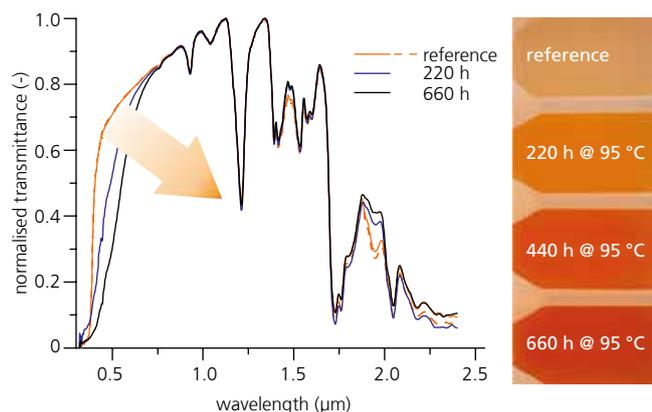
6 Optical characterization of the discoloration of polyamide test samples due to formation of chromophores during dry heat aging at 95 °C.
