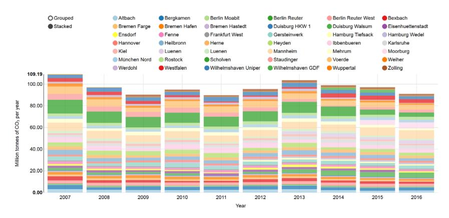
Releases to air. Pollutant Threshold: 0.1 Million tonnes of CO<sub>2</sub> per year. Graph: B. Burger, Fraunhofer ISE; Datasource: Umweltbundesamt (UBA), PRTR Register Source: https://www.energy-charts.de/emissions.htm?source=coal
