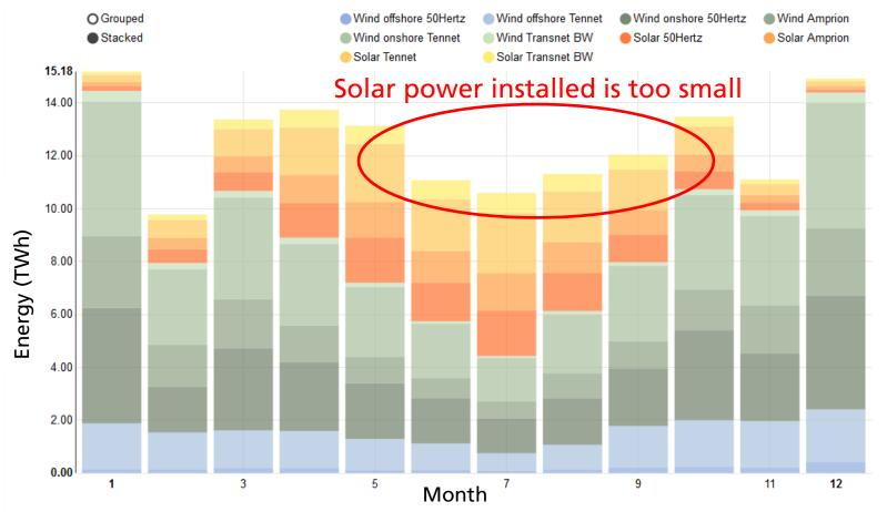
Despite high irradiation values in summer, solar power generation was too small to compensate for the collapse of the wind generation. The installed solar capacity is too small in relation to the installed wind capacity. Graph: B. Burger, Fraunhofer ISE; Source: <u>https://www.energy-charts.de/energy\_de.htm?source=solar-wind</u>
