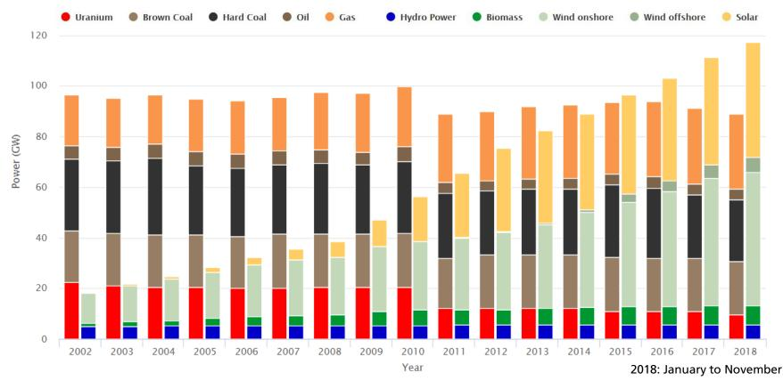
Since 2015, the installed power of renewables is greater than the installed power of fossil and nuclear. Graph: B. Burger, Fraunhofer ISE; Data: Bundesnetzagentur, Source: <u>https://www.energy-charts.de/power\_inst.htm</u>
