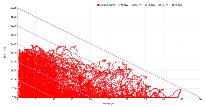
The graph shows approx. 35 thousand guarter-hour values of the solar output over the wind output in 2018. The maximum sum of solar and wind output was 53.3 GW on June 21 2018. 20.4 GW of this was attributable to solar and 32.9 GW to wind. This is only 53% of the installed capacity of 98 GW (43 GW Solar and 55 GW Wind).
