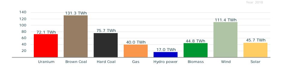
The chart shows the net electricity generation from power plants for the public power supply. Generation from power plants in the manufacturing, mining and quarrying industries, i.e. the self-generation of electricity in industry, is not included.
