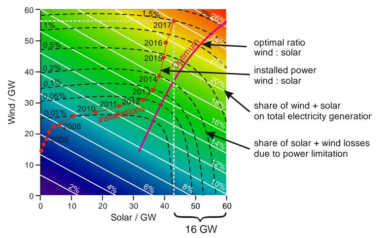
At the end of 2017, 16 GW of installed solar power was missing for the optimal ratio of wind to solar. Graph: B. Burger, Fraunhofer ISE
