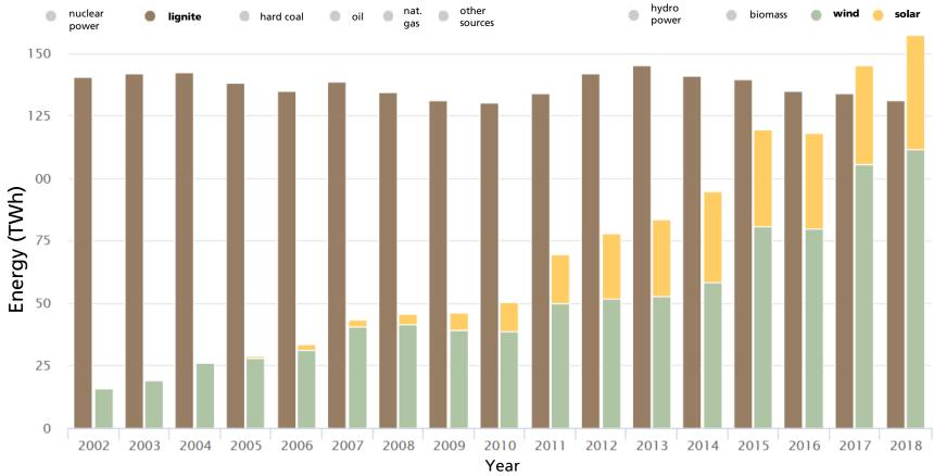
The total of solar and wind power generation was higher than lignite generation for the first time in 2017.
