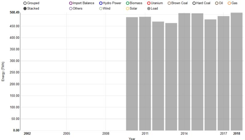
The load includes the electricity consumption and grid losses, but not the pump electricity consumption and the own consumption of conventional power plants.
