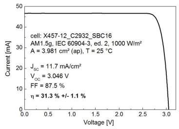
IV characteristic of the multi-junction solar cell with a new record efficiency of 31.3 %.  $\ensuremath{\textcircled{O}}$ Fraunhofer ISE
