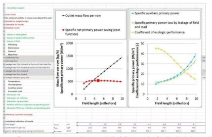
A small parameter study using "Aircow". Individual diagrams visualize the simulation results. ©Fraunhofer ISE
