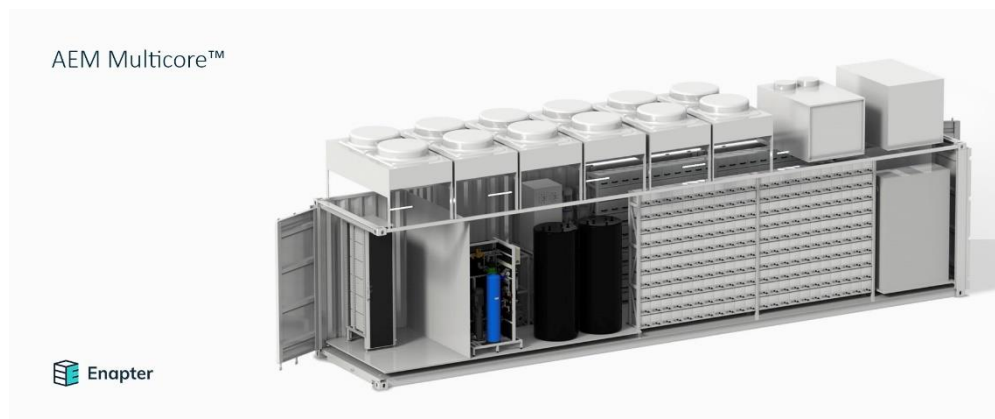
Figure 2-13: "Multicore" 1MW AEMEL system based on the modularization of 440 mass-produced AEM electrolysis core units by Enapter (courtesy of Enapter)
