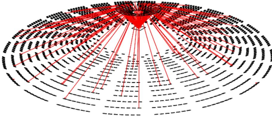
**Figure 12: Exemplary visualization with selected ray traces of Solar Tower Beam-Down system with a surrounding heliostat field**
