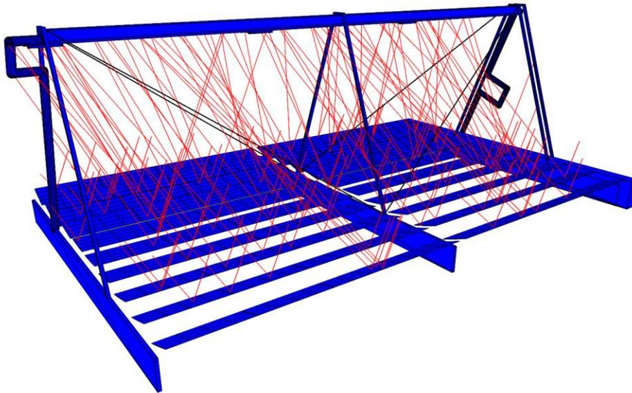
**Figure 9: Visualization of detailed simulation model including ray traces for a Linear Fresnel collector constructed at the premises of Fraunhofer ISE**
