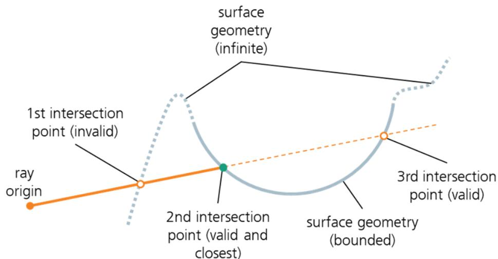
**Figure 3: Intersection point identification of ray (orange) with complex surface geometry (grey). The first intersection point is outside the surface boundaries and thus invalid. The second and third intersection points are both valid, yet the second intersection point (green) is closer to the ray origin and therefore selected.**
