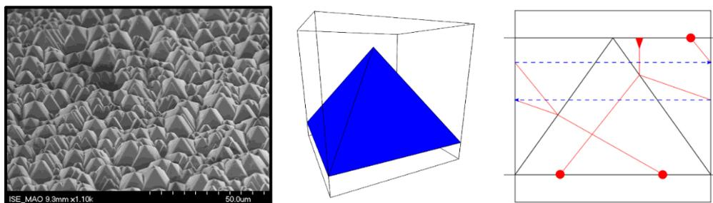
**Figure 7: Micro-textured surface with pyramid structures. Left: Microscopic photograph. Center: Visualization of a unit cell model, with periodic boundary conditions/teleport walls including randomization approach to account for pyramids of different size. Right: Side view of the scene, with depiction of a single ray. The blue dashed lines show the teleport behavior from left to right and vice versa.**
