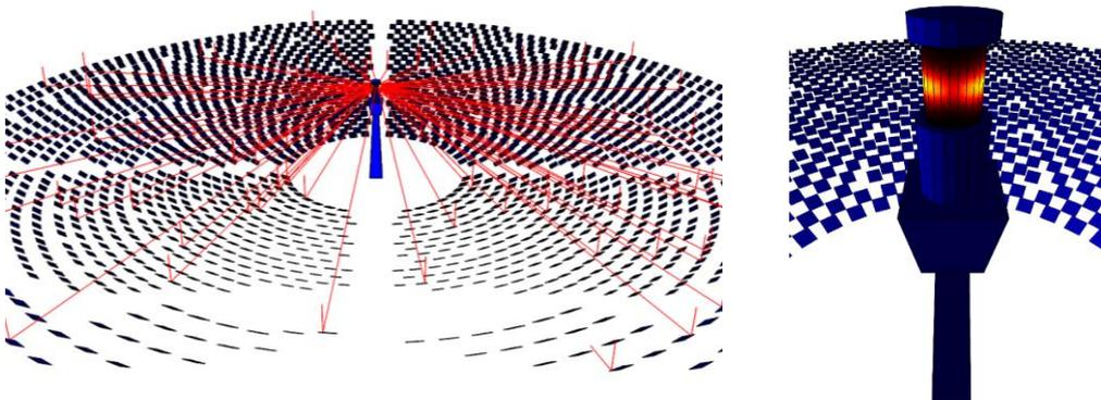
**Figure 11: Visualization with selected ray traces for the Solar Two system (formerly placed in the Mojave Desert, USA), including heliostat field, tower structure and receiver.**
