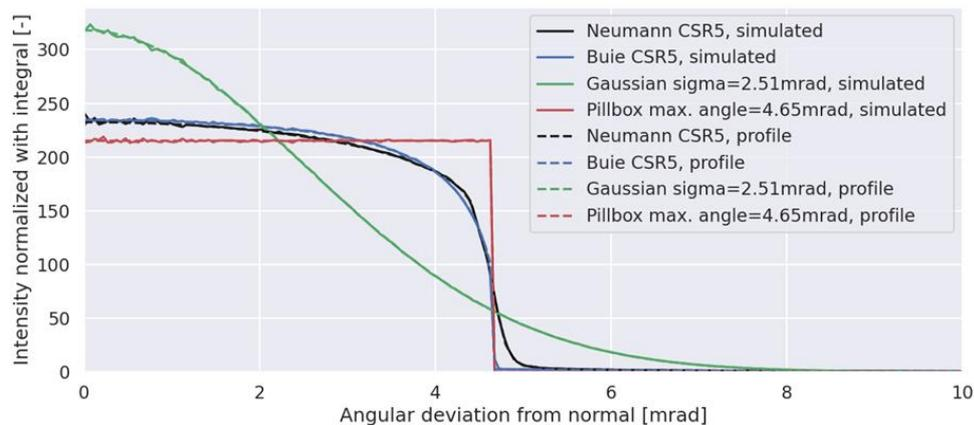
**Figure 4: Comparison of different sunshape profiles to represent direct solar beam irradiance and their equivalents from a radiometric simulation.**
