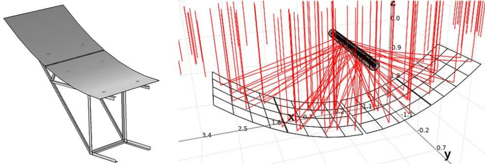
**Figure 10: Simulating the impact of gravity or wind-load induced deformations on optical collector performance. The simulation model includes a multi-faceted parabolic mirrors, the receiver glass envelope and the absorber tube. Local slope deviations are mapped on the mirror geometries (see 3.6).**
