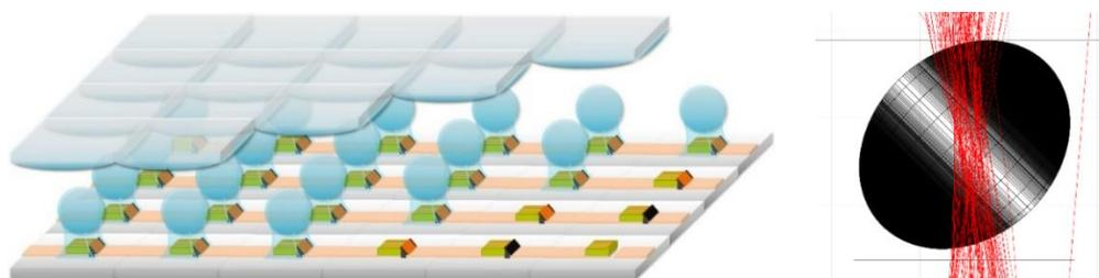
**Figure 8: Concentrator optics developed in the MicroCPV project. Different options for a Primary Optical Element (POE) are studied that concentrates the solar radiation onto a ball lens (Secondary Optical Element, SOE). Left: sketch of the MicroCPV module array. Right: Detail visualization of the ray paths in the SOE, which is – in order to study manufacturing tolerances – slightly non-spherical and skewed.**
