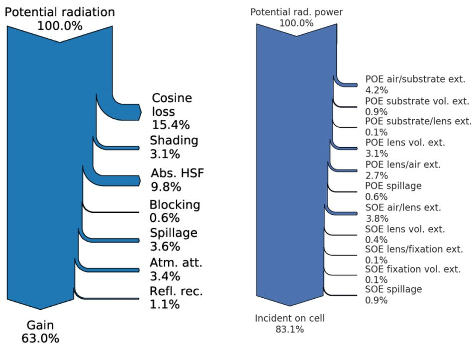
Figure 5: Detailed loss analysis based on evaluation of ray history. Left: exemplary annual analysis for a PS10-like polar heliostat field and cavity receiver (Abs. HSF=absorption on heliostat field, Atm. att.=atmospheric attenuation, Refl. rec.= Reflection from the receiver). Right: exemplary polychromatic analysis for a 2-stage (POE=primary optical element, SOE=secondary optical element) CPV system using refractory optics.
