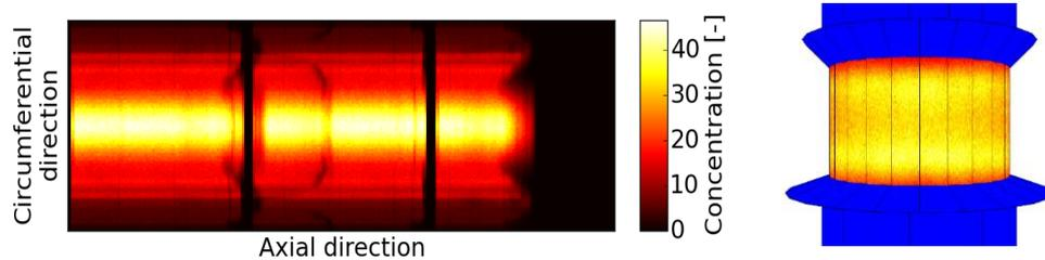
**Figure 6: Concentration distributions on regions of interest. Left: Concentration map on the absorber tube in a linear Fresnel collector, with the interaction of a secondary concentrator and shading from structural elements. Right: flux maps on the absorber panels of a surrounding external Solar Tower receiver with a secondary concentrator above and below the panels.**
