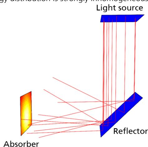
**Figure 1: Visualization of mock-up ray tracing scene: a light source with parallel rays, a scattering reflector with slope deviations and a discretized absorber with a concentration map. While only ten ray paths are depicted as red lines, the actual number of traced rays in this simulation – to yield the depicted concentration map – was larger than one million.**
