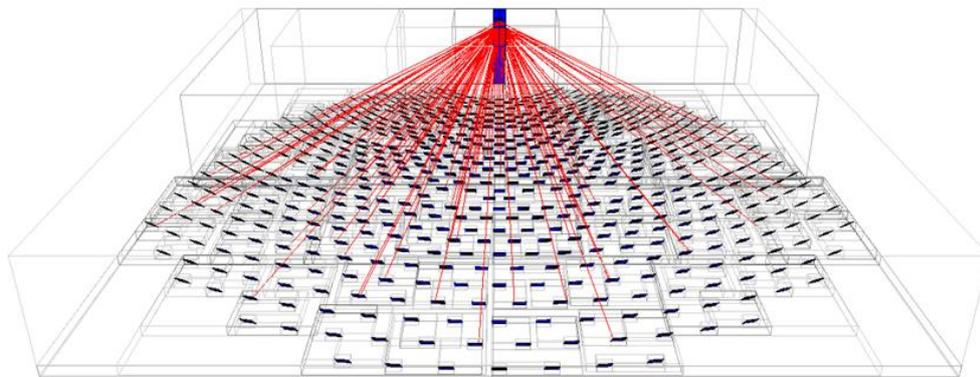
**Figure 2: Visualization of polar heliostat field and cavity receiver, showing automatically created, axis-aligned bounding boxes (light grey lines).**
