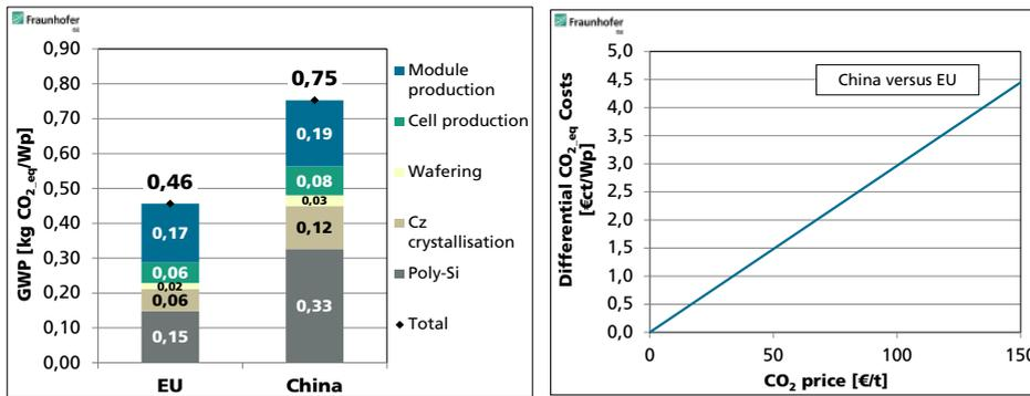
Carbon footprint of a Cz PERC glass-backsheet module production (left). Delta CO<sub>2</sub> cost of a Cz PERC module production located in Germany compared to China (right). Source: own calculations.
