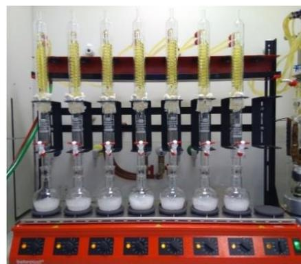
Figure 3: Serial extraction apparatus from Behrotest
