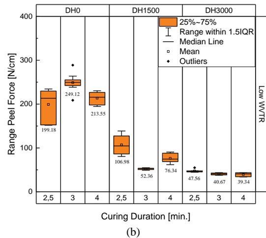
Figure 9: Peel force at the glass-encapsulant interface before and after DH1500 and DH3000 for (a) the 150 °C lamination process and the (b) 180 °C lamination process
