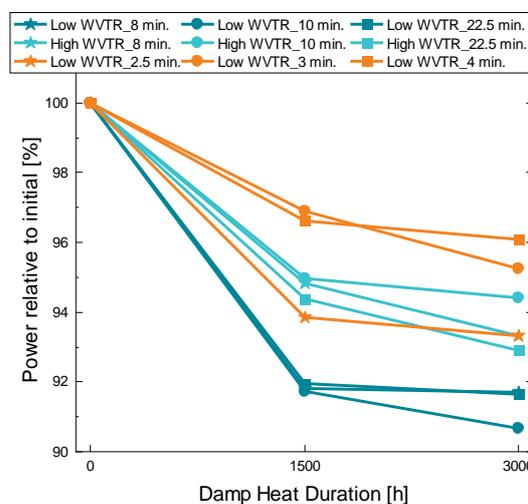
**Figure 5:** Module performances ratio before to after the DH test. Please note, that the orange curves are obtained
