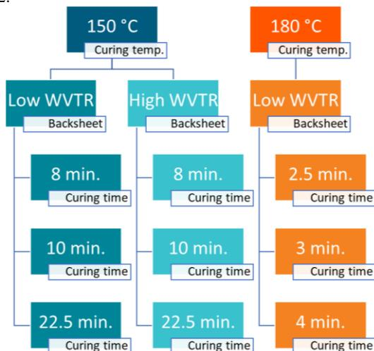
Figure 1: Lamination process specifications of the prepared samples
