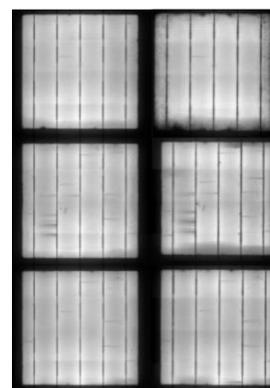
**Figure 7:** EL images of modules laminated with the 2.5, 3 and 4 min curing processes before and after DH3000
