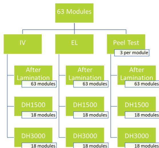
Figure 2: Module characterization methods and number of samples for each degradation condition
