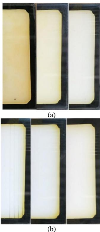
**Figure 6:** Discolouration of the 150 °C modules after DH1500, laminated at 8 min, 10 min and 22.5 min, respectively, (a) low WVTR backsheet, (b) high WVTR backsheet
