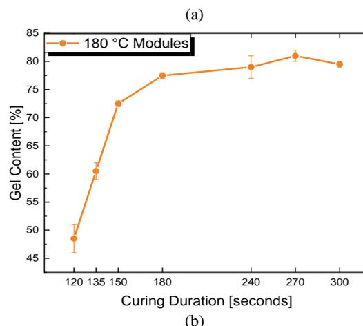
**Figure 4:** Gel content measurement results in samples manufactured using different process conditions, (a) 150 °C lamination temperature, (b) for 180 °C lamination temperature
