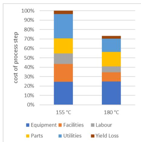
**Figure 10:** Cost structure of both lamination processes
