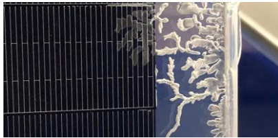
Figure 7: Features in encapsulation material abundant with PO-II samples after aTC200.
