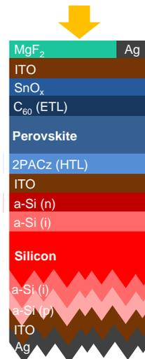
**Figure 1:** Layer stack of the perovskite-silicon tandem solar cell as published in [4].
