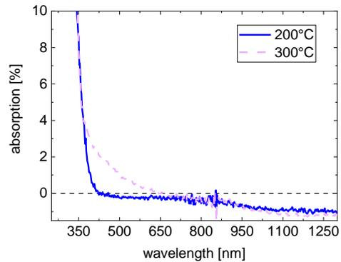
**Figure 2:** Calculated absorption of spray coated TiO<sub>x</sub> at substrate temperatures of 200 °C and 300 °C from transmission/reflection measurements.
