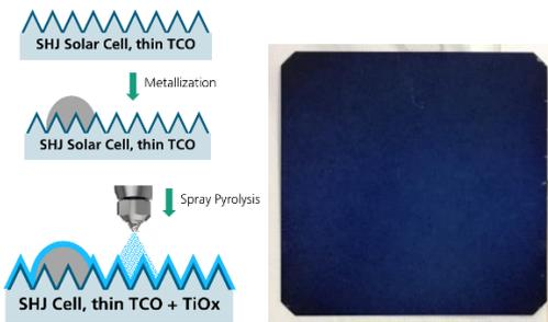
**Figure 4:** Top layers of the cells processed in this work (left), photograph of cell (without metallization, right)
