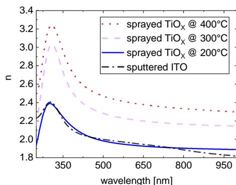
**Figure 3:** Refractive index  $n$  of spray coated TiO<sub>x</sub> thin films deposited on silicon at substrate temperatures of 200 °C, 300 °C and 400 °C; determined from SE measurements. For reference, the refractive index of a sputtered ITO is also included in the graph.
