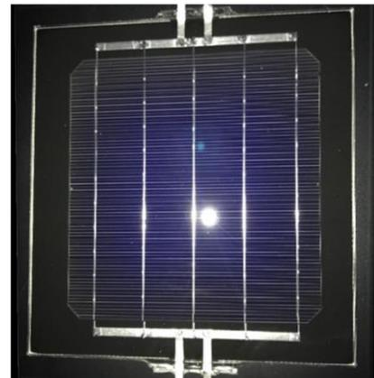
**Figure 5:** Photograph of single-cell-module fabricated from a M2+ SHJ solar cell with ITO/ $\text{TiO}_x$  layer stack.
