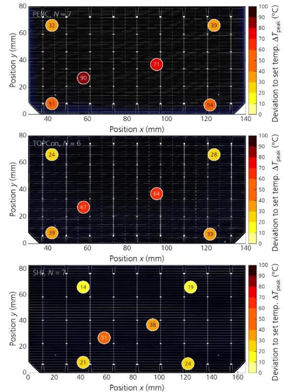
**Figure 6:** In-situ temperature measurement during IR soldering. Deviation of the measured mean peak temperature  $T_{peak}$  to the set temperature of soldering industrial PERC (top), TOPCon (middle) and SHJ (bottom) solar cells.
