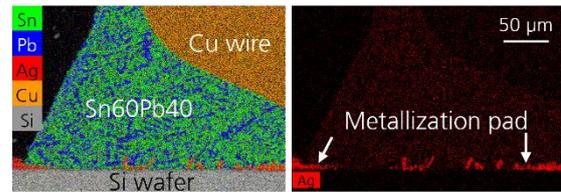
**Figure 4:** EDX cross section images of a solder joint on a very thin Ag pad on a Si solar cell. During soldering, Ag dissolves in the Sn matrix of the solder, leading to dissolution of the pad.
