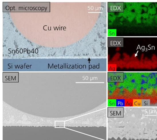
**Figure 3:** Cross section images of an ideal solder joint on a silicon solar cell. A diffusion zone and  $\text{Ag}_3\text{Sn}$  phase formation is found at the void-free interface between metallization and solder.
