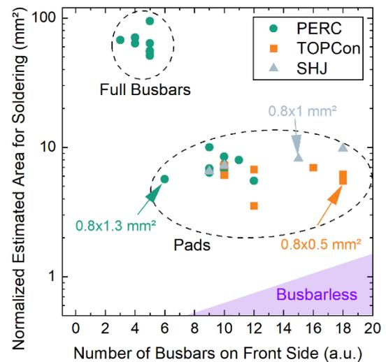
**Figure 1:** Normalized estimated area available for soldering depending on the number of busbars on the solar cell front side. As the solar cell format of the data points ranges from M6 to M12 the area is normalized to  $J_{sc}$  of 40 mA/cm<sup>2</sup>.
