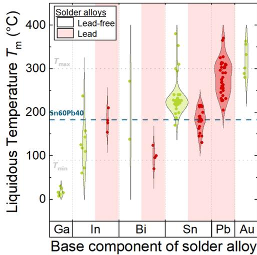
**Figure 5:** Liquidous temperature  $T_m$  of different solder alloys according to the main alloy component and divided between solar alloys containing lead and lead-free alloys.
