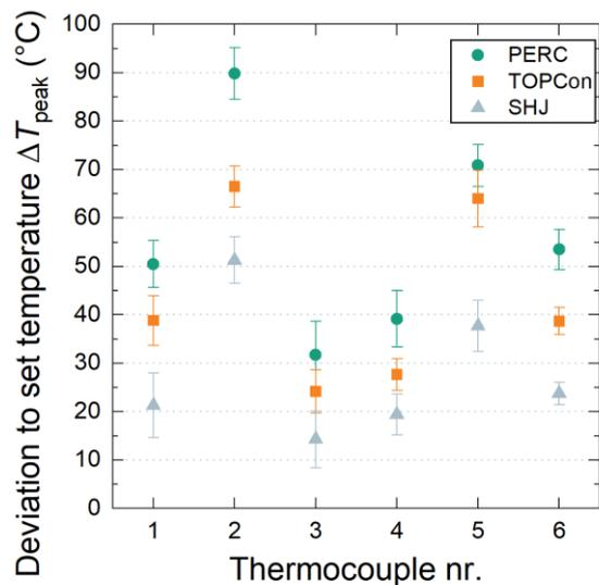
**Figure 7:** Measured peak temperature of solar cells at six different positions during IR soldering in an industrial stringer. Mean and standard deviation over min. 6 repetitions is given.
