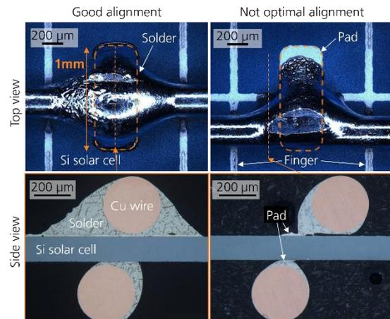
**Figure 2:** Top view and cross section microscopy images of soldered wires (0.32 mm) onto metal pads (width 1 mm) of a solar cell with good and not optimal alignment.
