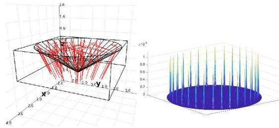
**Figure 3:** Ray tracing for a segmented cone at perpendicular incidence: visualization of the model (left) and the resulting reflectance distribution as polar plot (zenith angle radial, azimuth angle circular) (right).
