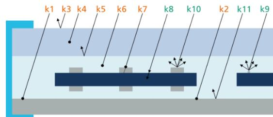
**Figure 4:** Schematic module cross-section illustrating the loss and gain mechanisms in the solar module.
