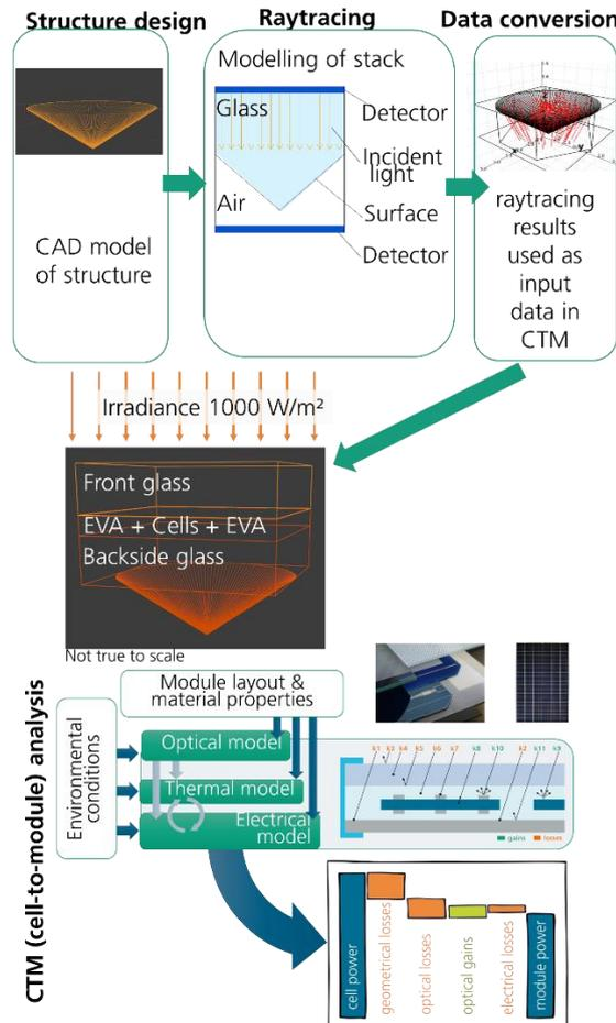
**Figure 2:** Schematic workflow of the simulation process to calculate the reflection gain for a structured backside glass, partly adapted from [7,8].
