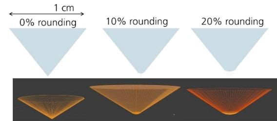
**Figure 6:** A sketch of the different rounded cones (top) and 3D images of the adapted cone structures with the different rounding (bottom).
