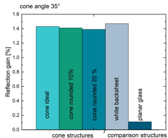
**Figure 7:** Reflection gain comparison for the ideal cone structure and for cones with different roundings compared to a white backsheet and a planar glass.
