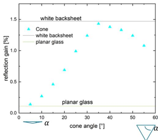
**Figure 5:** Results of the simulation study of the reflection gain for varying cone angle.
