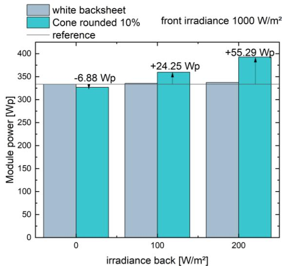
**Figure 8:** Module power for modules with either white backsheet or a structured glass with varying backside irradiance. The front irradiance is fixed at 1000 W/m<sup>2</sup>.
