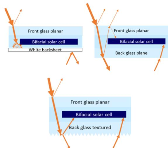
**Figure 1:** Cross-section views of the modules with different backsides and some possible light paths from the front and the backside: white backsheet (left), planar backside glass (middle), structured backside glass (right).
