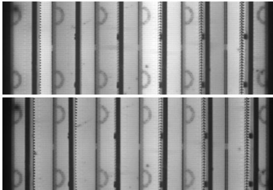
**Figure 5:** The upper EL image section of a M6 host cell shows clear signal fluctuations between the individual shingle cells. In the lower image, limiting resistors in the individual leads have improved the signal homogeneity.
