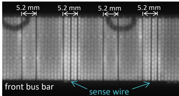
**Figure 3:** EL image of a shingle cell at a current of 10 A, which is 6 times  $I_{MPP}$  and clearly shows the series resistance effects.
