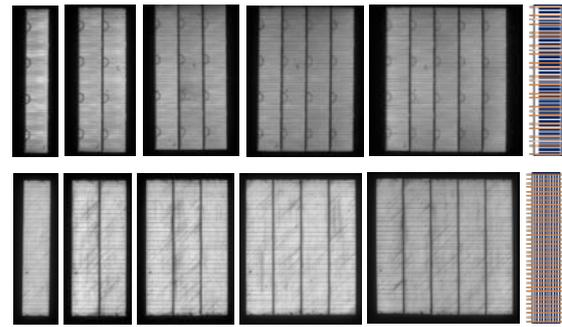
**Figure 6:** EL images of shingle cells with 25 wires running perpendicular to the busbars (top) and shingle cells with 35 wires running perpendicular to the fingers (bottom) during  $IV$  measurement. A contacting scheme is shown on the right side.
