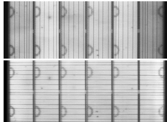
**Figure 4:** Sections of EL images of a section of the host cell ID 798 with 6 shingles contacted perpendicular to the fingers (top) and perpendicular to the busbars (bottom). The voltage distribution across the cell is significantly more homogeneous when contacting perpendicular to the busbars.
