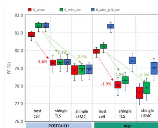
**Figure 9:** IV parameters of the host and shingle cells measured with (left) the PCBTOUCH unit and (right) the universal contact probes (ucp).
