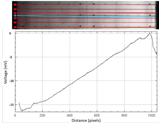
**Figure 2:** Top: EL image section of a solar cell that is contacted with the PCBTOUCH. The wires are only connected on the right side. Bottom: The voltage gradient was calculated from the grey value gradient of the EL image.
