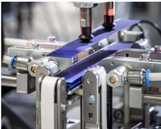
**Figure 1:** Shingle cells during magazine unloading. The blowing nozzles, which allow the cells to be separated in the magazine, are located to the right and left of the cell stack.
