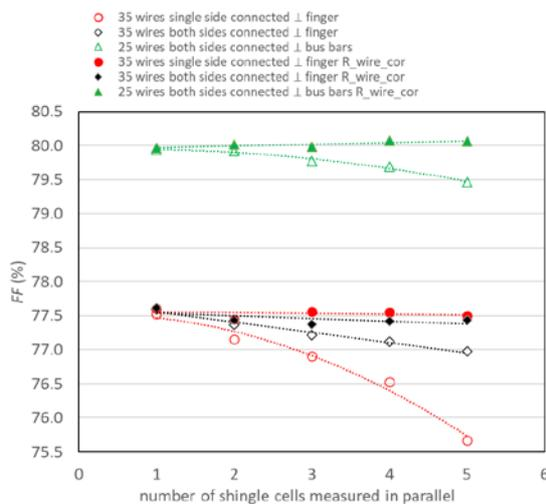
**Figure 8:** The measured  $FF$ s decrease in all test variants of contact configurations (see legend) with an increasing number of shingle cells measured in parallel (open symbols). If the series resistance contribution of the PCBTOUCH wires is considered (filled symbols), the  $FF$  remains almost at the same level with varying number of shingle cells measured in parallel.
