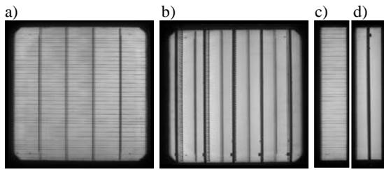
**Figure 7:** The EL images of (a-b) the M2 host cells and (c-d) the 1/5 shingle cells show the impact of contacting units. The host cells were contacted with (a) the PCBTOUCH unit perpendicular to the busbars and (b) the ucp stripes in the center of each of the shingle cells. The shingle cells were contacted using (c) the PCBTOUCH perpendicular to the busbar with 35 wires and (d) a centrally arranged ucp.
