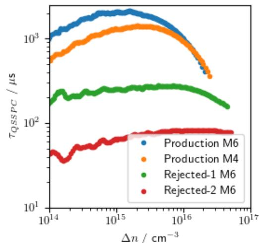
**Figure 4:** QSSPC lifetime vs. minority carrier injection level for the different production batches.
