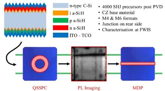
**Figure 1:** Layer stack of the textured SHJ precursors and process flow of the inline lifetime measurements. Wafers are placed onto the conveyor belt and automatically measured using QSSPC, PL imaging and MDP tools. The integration areas of the individual techniques are highlighted red in the sketch.
