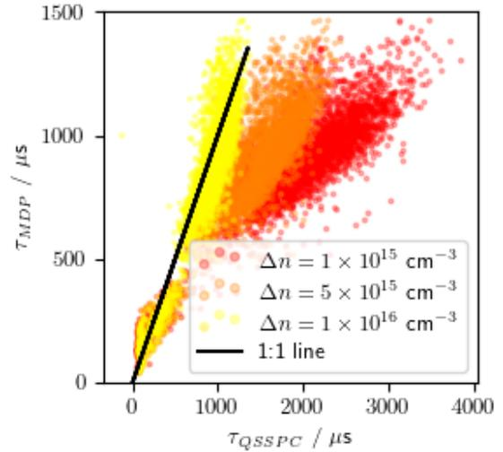
**Figure 5:** MDP lifetime plotted against QSSPC lifetime at different injection levels. The line of 1:1 proportionality is shown in black.
