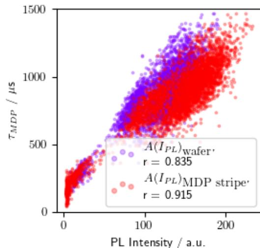
**Figure 6:** MDP lifetime plotted against different averagings of the PL intensity images. The blue and orange clouds, respectively, show the arithmetic mean  $A$  of each whole wafer, and a stripe matching the integration area of the MDP linescan.
