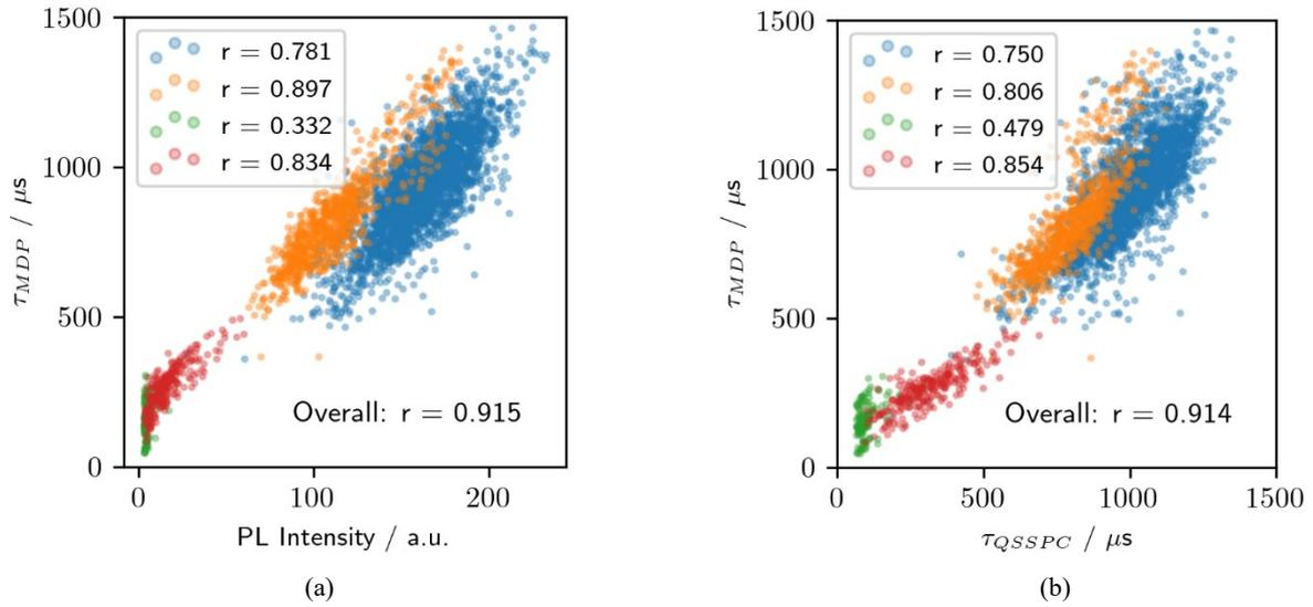
**Figure 2:** MDP lifetime (averaged over the full trace) plotted against (a) mean PL intensity and (b) QSSPC lifetime at  $1 \times 10^{16} cm^{-3}$  carrier density. The different coloured clusters correspond to the same groups as in Figure 3.
