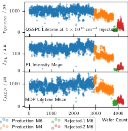
**Figure 3:** QSSPC (top), PL (middle) and MDP (bottom) data averaged for each wafer and plotted chronologically for 4164 SHJ precursors. Groups from different production batches are colour-coded.
