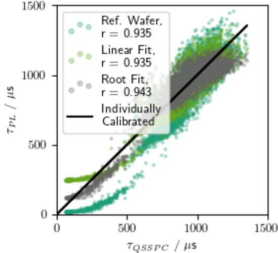
**Figure 7:** PL lifetime calculated via different methods of calibration against QSSPC.
