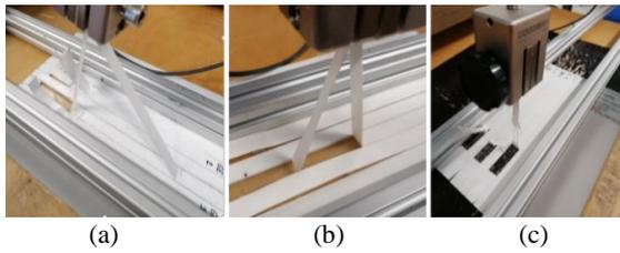
Figure 4: Photograph of the back sheet failure mode occurred during the peel test: Delamination of Backsheet in Sub-Layers (a), Delamination at the backsheet-encapsulant interface (b), and rupture of the Backsheet (c)
