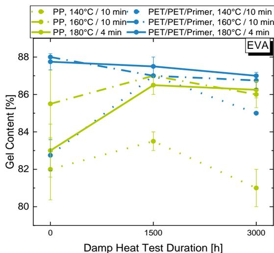
Figure 3: Gel-content of the EVA laminates with PP or with PET backsheet directly after lamination, after 1500 h and 3000 h damp heat test.
