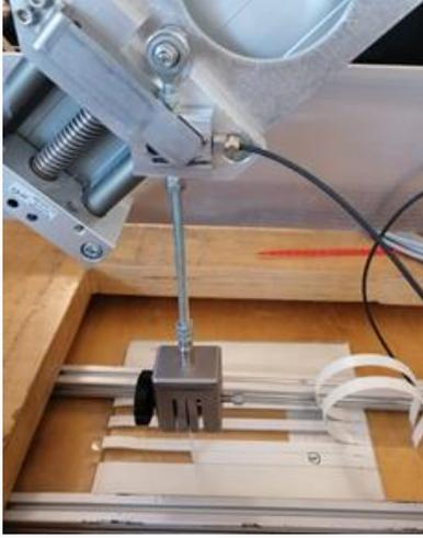
Figure 1: 90° Peel test at the glass-encapsulant interface
