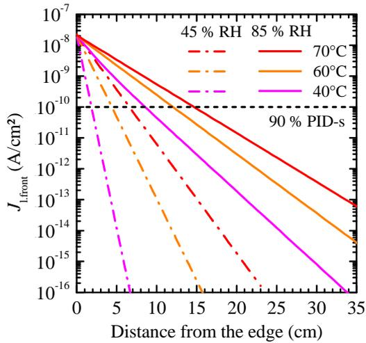
**Fig. 3:** Analytically calculated local leakage current density through the front side of a PV module with the cross-sectional layout 3.2 mm glass/0.42 mm EVA/cell array. The bias voltage between cell array and grounded module is 1000 V. The dashed black line indicates the expected local 90 % power degradation of PID-s prone c-Si solar cells after 6.9 days.
