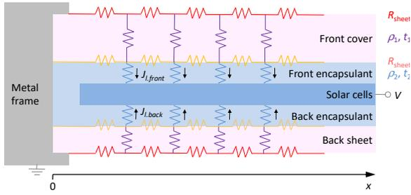
**Fig. 1:** Schematic drawing of a c-Si PV module cross section showing leakage current paths and electrical material and interface parameters.
