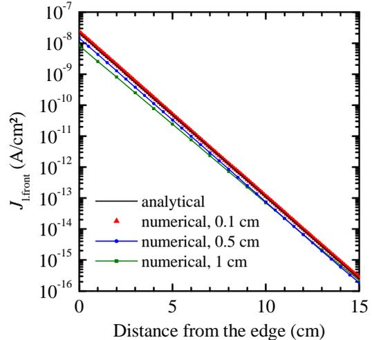
**Fig. 2:** Comparison of analytically and numerically calculated leakage current density through the front side of a PV module. The numbers in the legend indicate the node distances in the numerical simulation.
