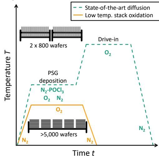
**Figure 1:** Schematic illustration of the state-of-the-art tube furnace  $\text{POCl}_3$  diffusion process as a function of the temperature  $T$  over time  $t$  with a typical process throughput of 1,600 wafers (M6 configuration). Further, the low temperature stack oxidation (LoTSOx) with a throughput of more than 5,000 wafers is illustrated.
