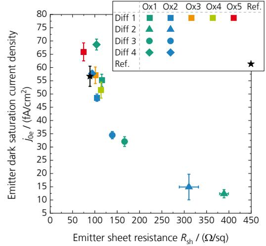
**Figure 4:** Emitter dark saturation current density  $j_{0e}$  on textured surfaces after  $\text{SiO}_2/\text{SiN}_x$  passivation and firing as a function of the emitter sheet resistance  $R_{sh}$ .
