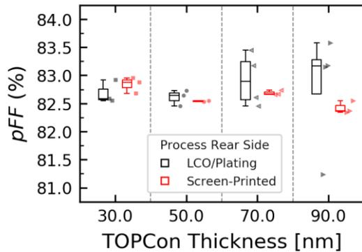
**Figure 6:** Pseudo-fill-factor  $pFF$  measured for the cells.
