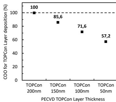
**Figure 2:** Normalized cost of ownership (COO) for the PECVD TOPCon process with decreasing TOPCon layer thickness. The typical thickness as used for screen-printing on TOPCon is in the range of 100 to 200 nm. Taken from [5].
