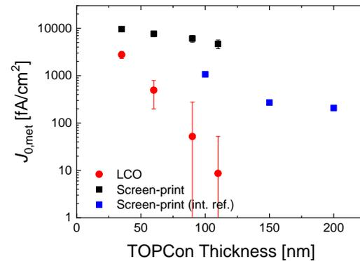
**Figure 3:**  $J_{0,met}$  for LCO in comparison to screen-printed contacts for a variation of the TOPCon thickness in comparison to screen-printed references. In addition the values for screen-printed contacts for a second batch (internal reference) is given, for which the values were a bit lower but still significantly higher than for LCO.
