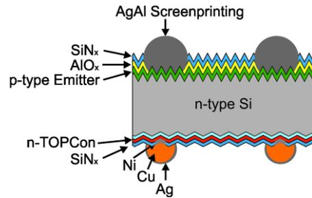
**Figure 4:** Sketch of the investigated cell design. The cell features a boron emitter at the front, passivated by an Al<sub>2</sub>O<sub>3</sub>/SiN<sub>x</sub> stack. The rear is passivated by a TOPCon/SiN<sub>x</sub> stack. The rear contacts are realized either by screen-printing or by NiCuAg plating. The front contacts are always realized by screen-printing.
