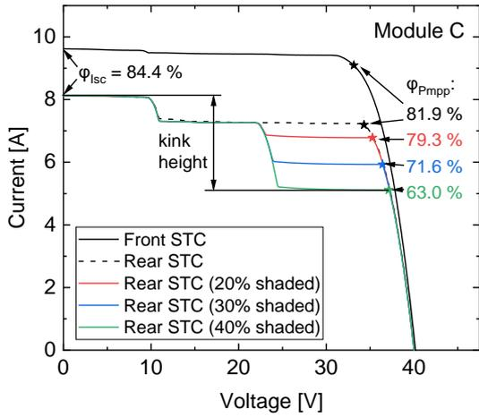
**Figure 7** Front and rear  $I$ - $V$  curves of module C at STC for different amount of rear shading. Stars indicate maximum power points. The relative difference between  $I_{sc, rear}$  and  $I_{mpp, rear}$  is referred to as kink height.
