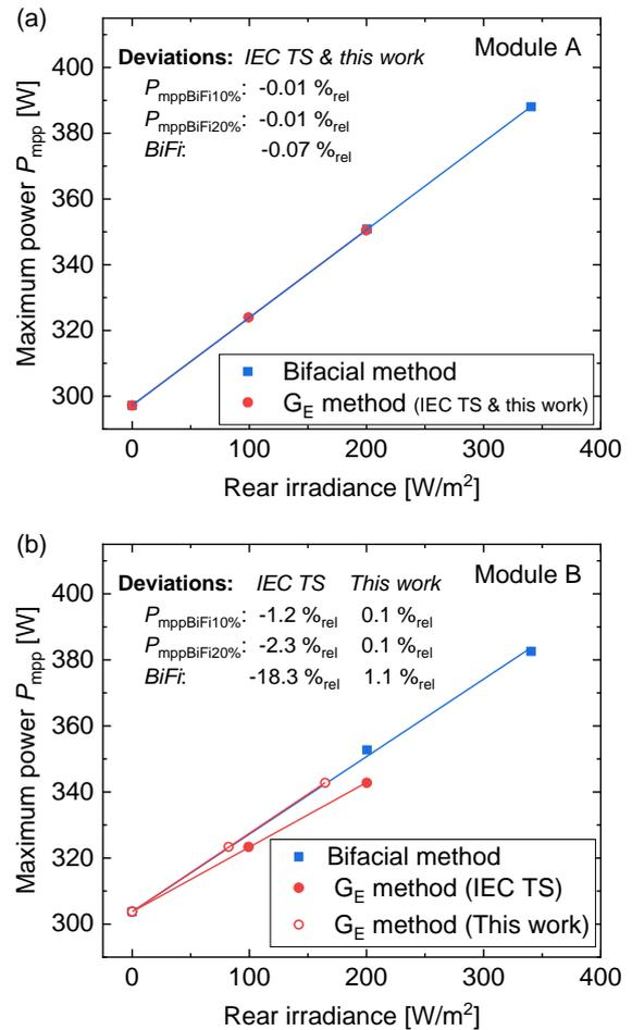
**Figure 6:** Measured maximum power  $P_{\text{mpp}}$  for different rear irradiance levels with both-sided illumination (blue squares) or with front-side illumination only using the  $G_E$  method (orange circles) for the two bifacial solar modules of Figure 5. The deviations in the standardized parameters  $P_{\text{mppBiFi10\%}}$ ,  $P_{\text{mppBiFi20\%}}$  and  $BiFi$  between the  $G_E$  and bifacial methods are given in the tables in the figures.
