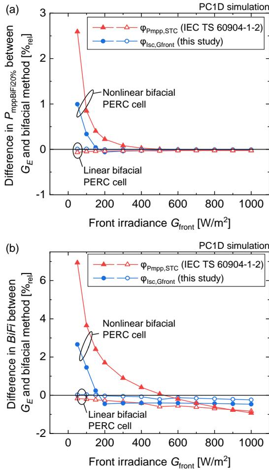
**Figure 4:** PC1D-simulated difference in the parameters (a)  $P_{mppBiFi20\%}$  and (b)  $BiFi$  between the  $G_E$  and the bifacial methods as a function of front irradiance for the two different approaches of  $\varphi$  evaluation: the IEC TS approach (red triangles) and the approach proposed in this study (blue circles).
