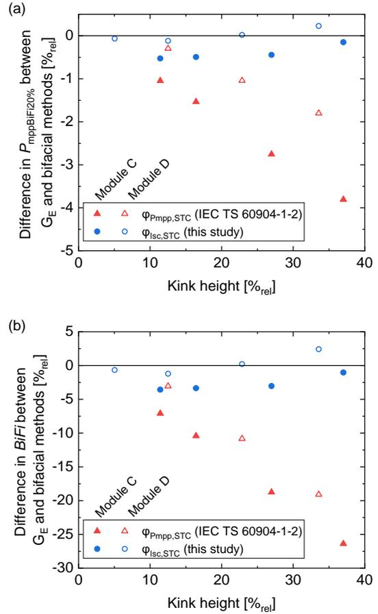
**Figure 9:** Deviation in (a)  $P_{mppBiFi20\%}$  and (b) *BiFi* between  $G_E$  and bifacial methods as a function of the kink heights in the rear  $I-V$  curves, which is quantified by the difference between  $I_{mpp,rear}$  and  $I_{sc,rear}$ , for modules C and D. Red triangles represent the  $\varphi$  evaluation of IEC TS 60904-1-2, blue circles represent the evaluation proposed in this study.
