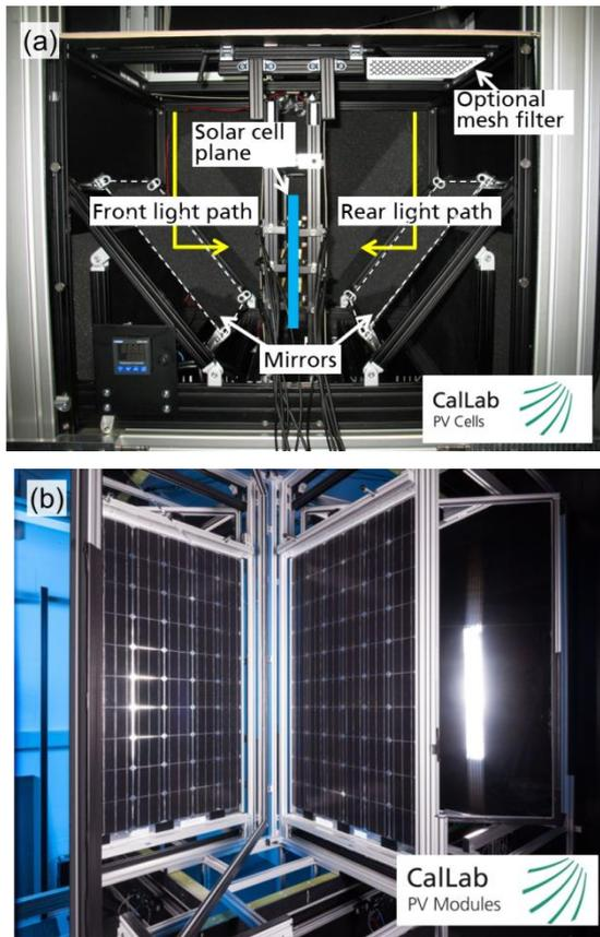
**Figure 2:** Pictures of two-mirror setups used in this study for the  $I$ - $V$  measurement of (a) bifacial solar cells and (b) bifacial solar modules.
