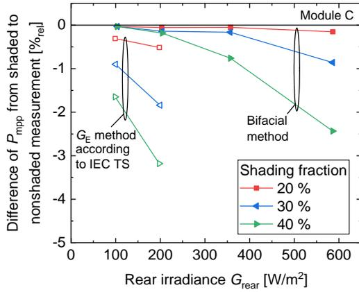
**Figure 8** Deviation in  $P_{mpp}$  between shaded to nonshaded measurement for different rear irradiance levels measured with bifacial method (full symbols) and  $G_E$  method according to the IEC TS (open symbols). Measurements with the  $G_E$  method as proposed in this study are not shown as  $P_{mpp}$  is not affected by rear shading.
