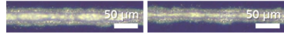
Figure 4: Microscope images of the screen-printed fingers after contact firing for (left) group Ref with 33 \mu\text{m} screen opening and (right) group Gr1 with 24 \mu\text{m} screen opening.
