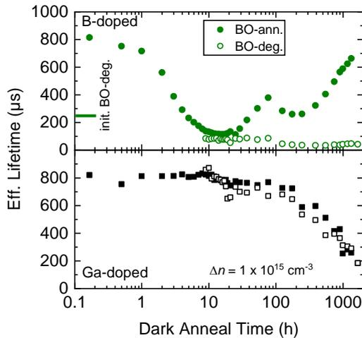
Figure 1: Effective carrier lifetime extracted at  $\Delta n = 10^{15} \text{ cm}^{-3}$  during dark anneal at  $175^\circ\text{C}$  of B-doped (top graph) and Ga-doped (bottom graph) samples in the BO-annealed (closed symbols) and BO-degraded (open symbols) states.
