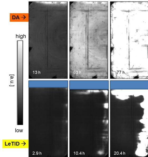
Figure 3: Progress of regeneration during dark anneal (upper row, BO-annealed state) compared to LeTID at 1 sun eq. (lower row) of two halves of the same B-doped wafer. All PL images were taken at a generation equivalent to 0.1 sun and scaled the same. During the measurements of the LeTID samples, the upper edge was masked in order to minimize the overflow of the camera detector (blue rectangles).
