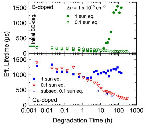
Figure 2: Effective carrier lifetime extracted at  $\Delta n = 10^{15} \text{ cm}^{-3}$  during illuminated anneals at  $75^\circ\text{C}$  of B-doped (top graph) and Ga-doped (bottom graph) samples illuminated with 1 sun eq. (closed symbols) and 0.1 sun eq. (open symbols), respectively.
