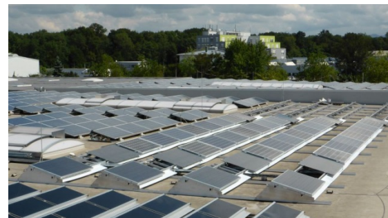
Figure 1: View of the test field. Each of the 4 rows carries 9 modules under test. The leftmost modules are additional reference modules provided by Fraunhofer ISE.
