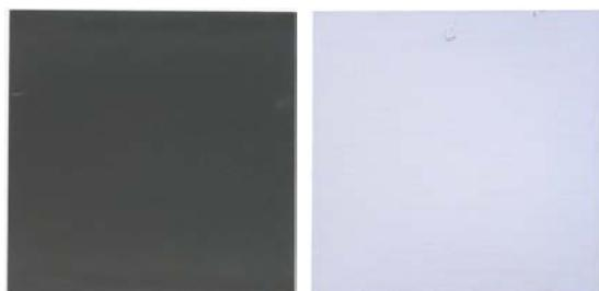
**Fig. 6:** Photos of the front (left) and the rear sides (right) of a 6 inch CZ Si wafer after alkaline texturing. The rear side was protected by an APCVD SiO<sub>2</sub> layer, which was subsequently etched in HF.
