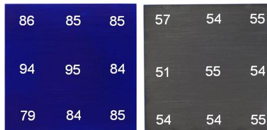
**Fig. 3:** Photos and SiO<sub>2</sub> thickness map of the upper side (left) and lower side (right) of a smooth 6 inch CZ Si wafer. The wafer was placed during APCVD of SiO<sub>2</sub> at a distance of 55 mm from the bottom plate.
