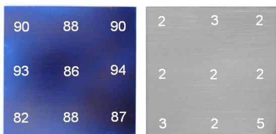
**Fig. 2:** Photos of a smooth 6 inch CZ Si wafer after APCVD of SiO<sub>2</sub> at room temperature showing the film thickness in nm measured by ellipsometry. **Left:** Upper wafer side. **Right:** Lower wafer side that was positioned on the base plate of the deposition chamber. Note that the horizontal lines visible in the photos are reflections of saw marks on the wafers and are not correlated with the APCVD process.
