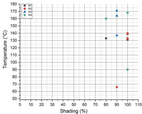
**Figure 7:** Approach 3 – three cells per module shaded on the rear side. For high-shunt resistance cells, the highest temperatures are typically measured at shading levels > 80 %.
