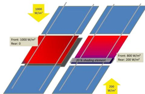
**Figure 2:** Schematic representation of a shaded bifacial cell. Left string: the rear side of a cell is fully shaded; right string: the front side is 20 % shaded. Assuming a bifacial factor of 1, the amount of dissipated energy is similar in both cases.
