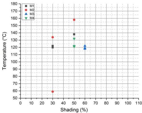
**Figure 6:** Approach 2 – three cells per module shaded on the front side. For high-shunt resistance cells, the highest temperatures are typically measured at shading levels < 60 %.
