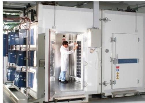
**Figure 3:** Test setup with mounted module
