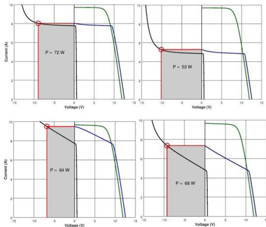
**Figure 1:** Simplified I-V curve of a cell string of 20 cells with one cell shaded to 80 % (left) and 50 % (right) irradiance compared to the others, with the shaded cell assumed to have high (top) or low (bottom) shunt resistance. Legend: **Green:** unshaded cells; **Black:** shaded cell; **Blue:** resulting curve; **Gray area:** dissipated energy
