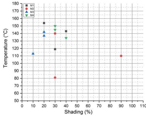
**Figure 5:** Approach 1 – three cells per module shaded on the front side. For high-shunt resistance cells, the highest temperatures are typically measured at shading levels < 40 %.
