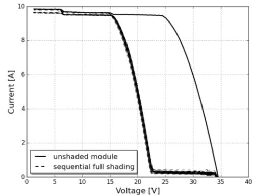
**Figure 4:** Exemplary I-V curves of a module with fully shaded cells and none of the cells indicating low shunt resistance.
