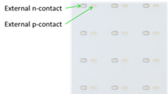
Figure 6: Rear view of an all-purpose MWT solar cell segment with 12 external n and p contacts
