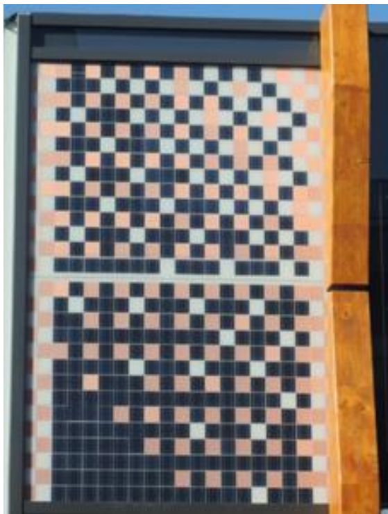
Figure 10: Façade mock-up of mosaic PV modules with different designs and solar cell coverage; top module: 119 AP-MWT cells (38.9% of area photovoltaically active); bottom module: 167 AP-MWT cells (55.0% of area photovoltaically active).
