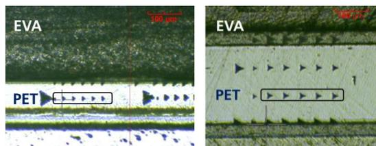
**Figure 5:** Microscopic images of the cross-section of the laminates after indentations on the BS1 (left) and BS2 (right) as laminated in glass/EVA/BS stack and aged under DH conditions. The values of the five indents on the same plane are averaged.
