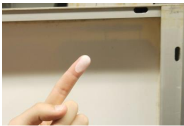
Figure 1: Finger with white powder from chalking backsheet
