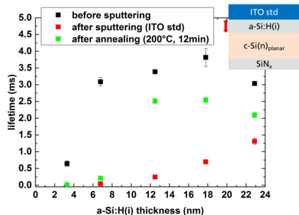
**Figure 2:** Minority charge carrier lifetimes for various a-Si:H(i) layer thicknesses before (black squares) and after (red squares) ITO deposition and a subsequent annealing (green squares).
