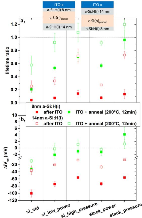
**Figure 5:** Normalized mc lifetimes (a) and change in  $iV_{oc}$  (b) during sputtering and annealing for five ITO deposition recipes (listed in Tab. 2) applied on a-Si:H(i) passivation layers of 8 nm (filled squares) and 14 nm (empty squares) thickness.
