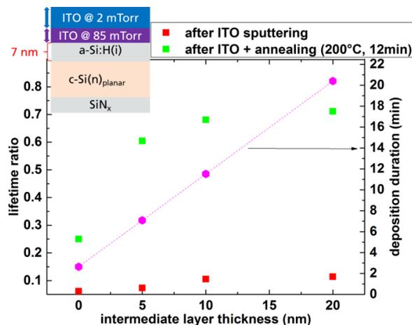
**Figure 7:** Influence of the thickness of the gently deposited protective ITO layer on the sputter-induced degradation and the process duration of the entire ITO film. The soft layer was deposited at 85 mTorr and 200 W, before the remaining ITO to build a 75 nm thick film followed under standard conditions (2 mTorr, 200 W).
