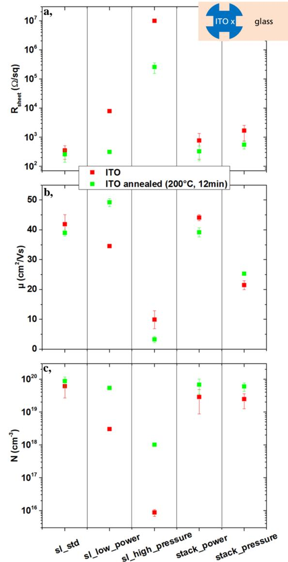
**Figure 6:** Electrical film properties sheet resistance (a), charge carrier mobility (b) and concentration (c) of 75 nm thick ITO deposited on glass according to the recipes in Tab. 2 and subsequent to an annealing step at 200 °C, measured via the van der Pauw method.
