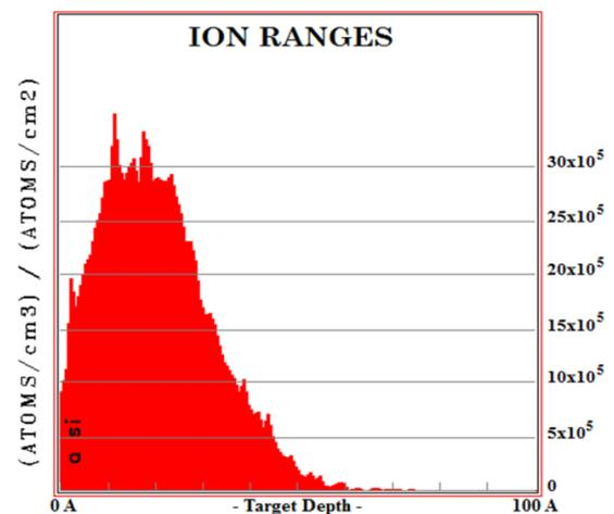
**Figure 1:** SRIM Monte Carlo simulation for the penetration depth of oxygen atoms with an initial kinetic energy of 252 eV in a-Si:H. The amount of oxygen atoms within a cubic centimeter of a-Si:H, normed by the number of impacting particles per area, is shown for a depth of up to 100 angstrom below the surface.
