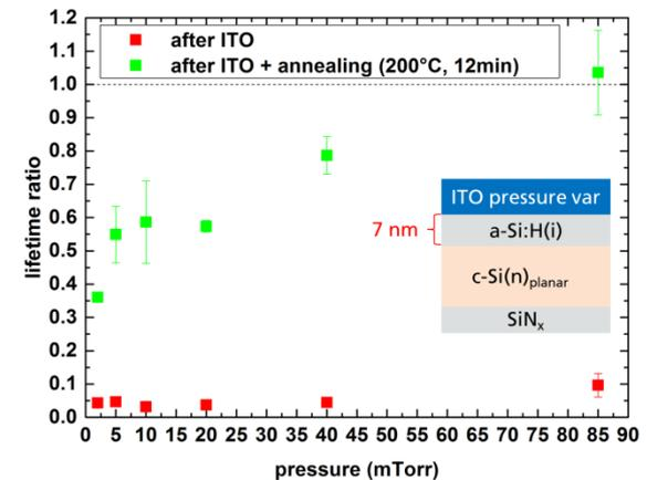
**Figure 4:** Minority carrier lifetimes after ITO sputter processes at various chamber pressures and subsequent to annealing. The values are normalized by the individual initial pre-sputter mc lifetime (at a level of 1.5 ms) to simplify comparison.
