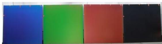
**Figure 1:** Full-area coating of module front glass cover [11]
