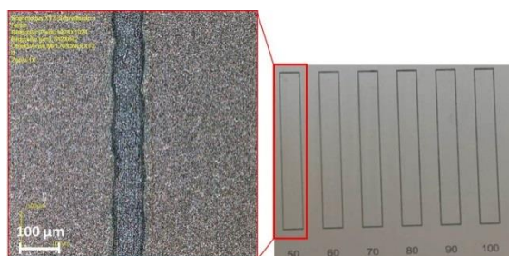
Figure 8: Results of ESP on 100 nm PVD-Al layer with \text{NaNO}_3 -based paste; Photograph of etched structures by using 50 \mu\text{m} to 100 \mu\text{m} screen openings (right); microscope image of etched structure with a line width of 80 \mu\text{m} aluminum achieved with 50 \mu\text{m} screen opening (left)
