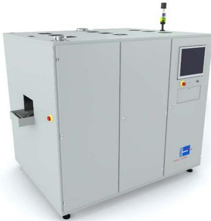
**Figure 6:** Prototype of single track inline regeneration tool based on UFR technology. It offers a belt speed of up to 8000 mm/min and a footprint of less than 4 m<sup>2</sup>.
