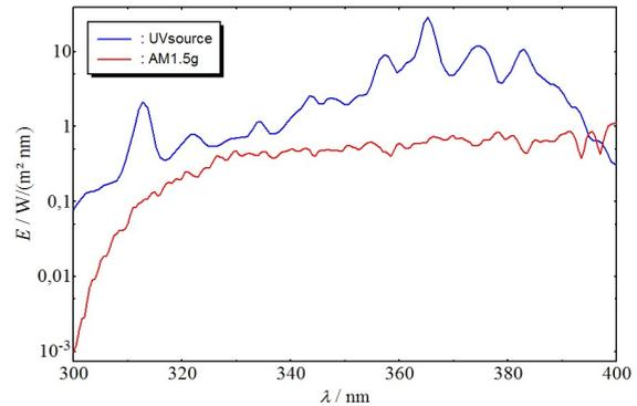
**Figure 2:** Comparison of the spectral irradiance of the Labino UV-light source and AM1.5g.
