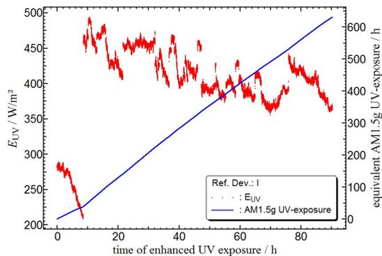
**Figure 3:** Monitoring the UV-irradiance during degradation by measuring the photocurrent.
