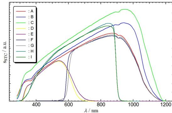
**Figure 1:** Spectral responsivity of the investigated reference devices. The assignment A-I can be found in Table 1.
