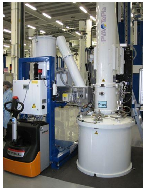
Figure 4: Mobile Recharge System docked on Cz-puller
