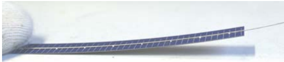
Figure 9: Cell section after cooling to 20 °C for bow measurement using the set up shown in figure 10
